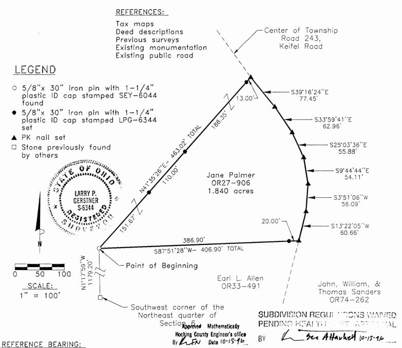
The West line of the Northeast quarter of Section 6 as North 1 degree 17 minutes 59 seconds West. Bearings are based upon an assumed meridian and are to denote angles only.
