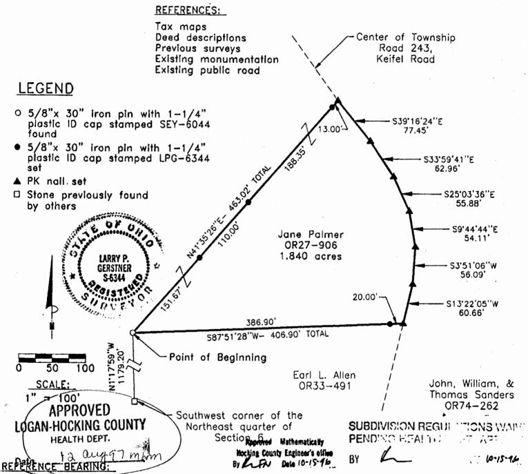
The West line of the Northeast quarter of Section 6 as North 1 degree 17 minutes 59 seconds West. Bearings are based upon an assumed meridian and are to denote angles only.
