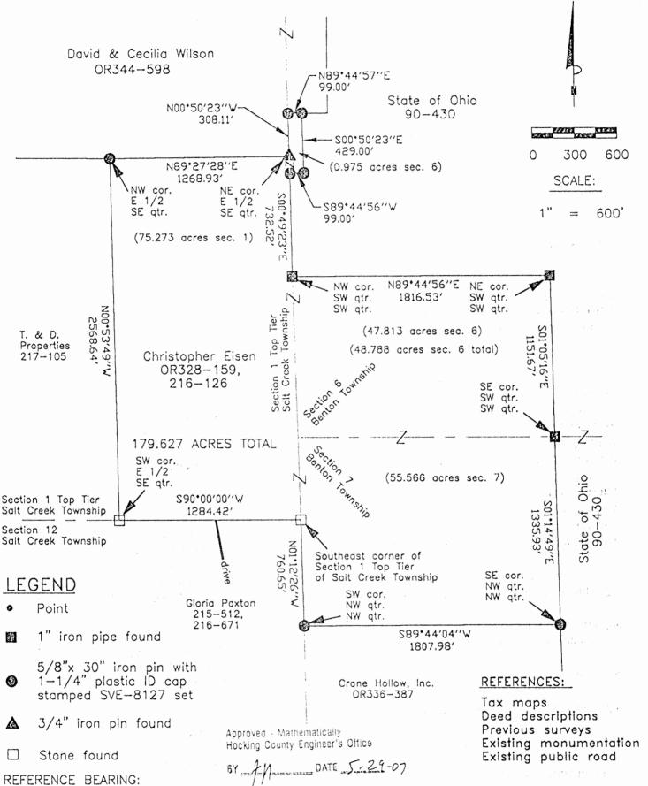
The south line of Section 1 Top Tier of Salt Creek Township as South 90 degrees 00 minutes 00 seconds West. Bearings are based upon an assumed meridian and are to denote angles only CERTIFICATION:
