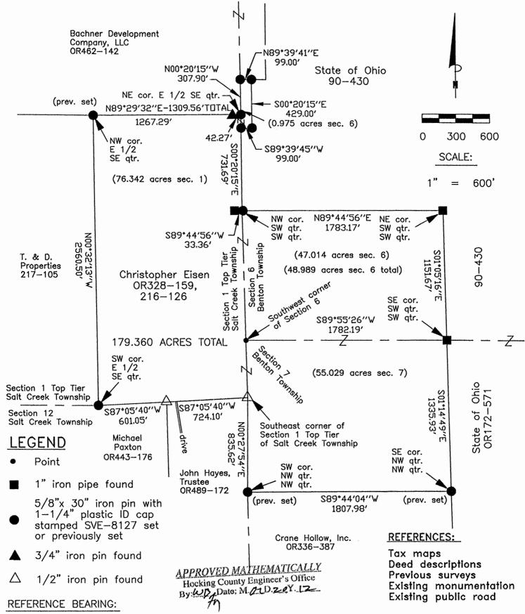
The south line of Section 1 Top Tier of Salt Creek Township as South 87 degrees 05 minutes 40 seconds West. (Established by R.M. Sharrett Survey June 1989). Bearings are based upon an assumed meridian and are to denote angles only.
