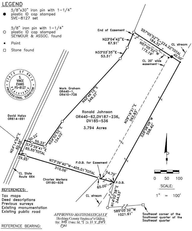
The south line of Section 17 as South 85 degrees 05 minutes 32 seconds West. Bearings are based upon an assumed meridian and are to denote angles only.
