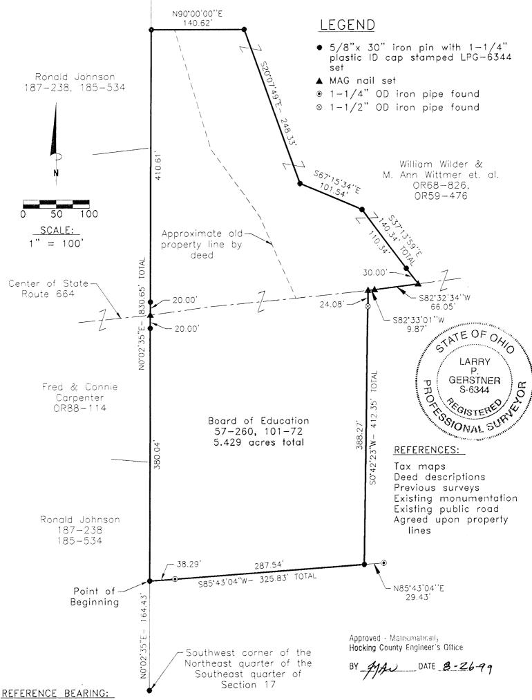
The East line of Section 17 as South 0 degrees 00 minutes 00 seconds East. Bearings are based upon an assumed meridian and are to denote angles only. <u>CERTIFICATION:</u>
