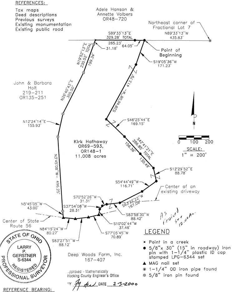
The East line of Section 21 as South 0 degrees 28 minutes 54 seconds West. Bearings are based upon an assumed meridian and are to denote angles only.
