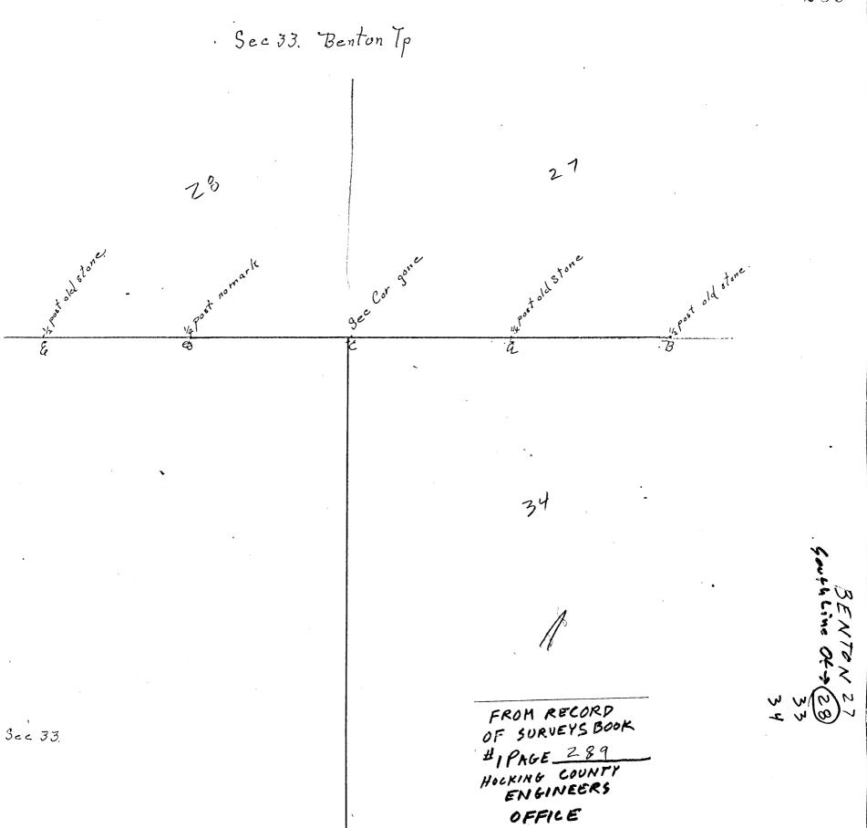
At request of Wilber Turner made survey to mark the Sec Line Between Secs 28433 who the Etof NE to of Sec 33. Found old Stones at a &B. Ran Line to E. Mised E. & feet. Corrected line. Placed Cat's way between B &E. Placed Dat & way between CDE.
