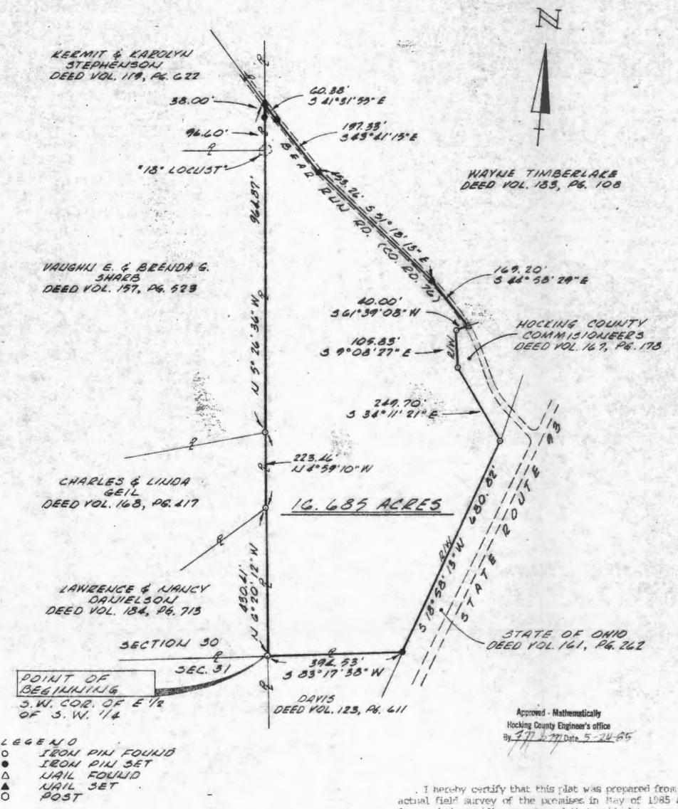
The bearing system for this plat is based on the right of way plans for State Route 93, the parcel; for which are recorded in Deed Vol. 161, Pg. 262 and Deed
