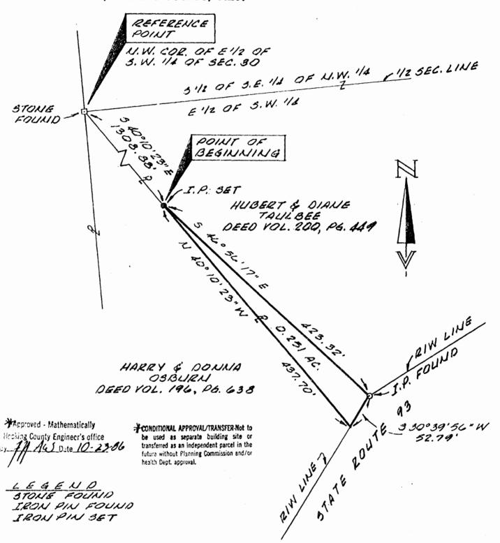
The bearing system for this plat is based on the right of way plans for State Route 93, the description for which is recorded in Deed Volume 161, Page 262.
