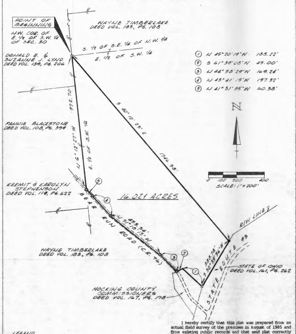
The bearing system for this plat is based on the right of way plans for State Route 93, the description for which is recorded in Deed Vol. 161, Pg. 262.
