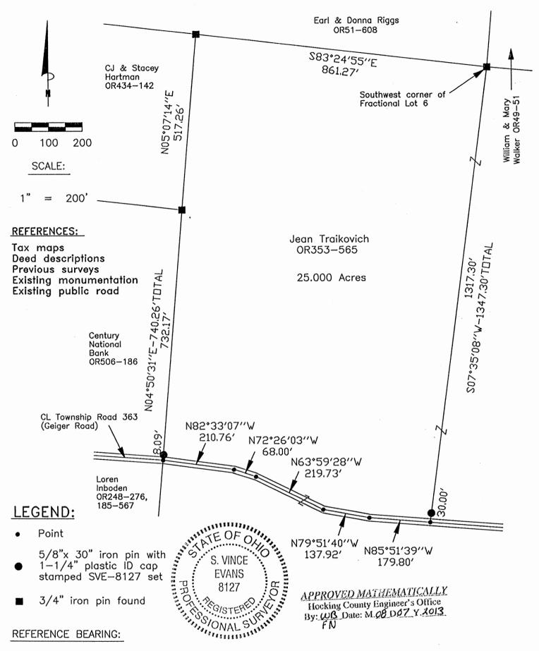
The south line of Fractional Lot 6 as South 84 degrees 34 minutes 07 seconds East. Bearings are based upon an assumed meridian and are to denote angles only.
