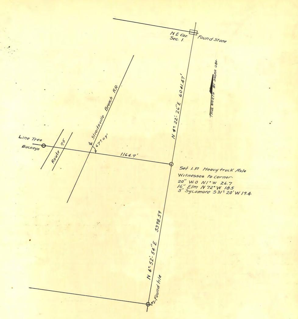
I certify that I have Placed an iron pin at the South East Corner Section I Falls twp. in accordance with an old Survey found in Vol. 123 Straitsville Branch of the C.& O. R.R. Under date of 1879. Ond filed in office of Valuation Eng. C.& O. R.R. Spahr Bldg. Columbus, Ohio.
