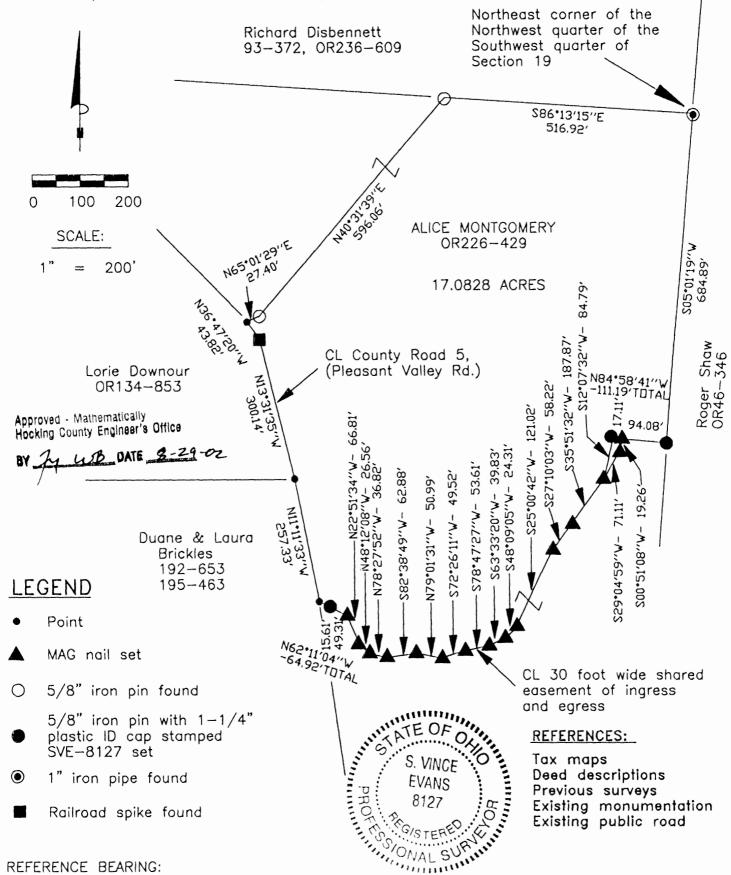
The East line of the Northwest quarter of the Southwest quarter of Section 19 as South 05 degrees 02 minutes 02 seconds West. Bearings are based upon an assumed meridian and are to denote angles only.
