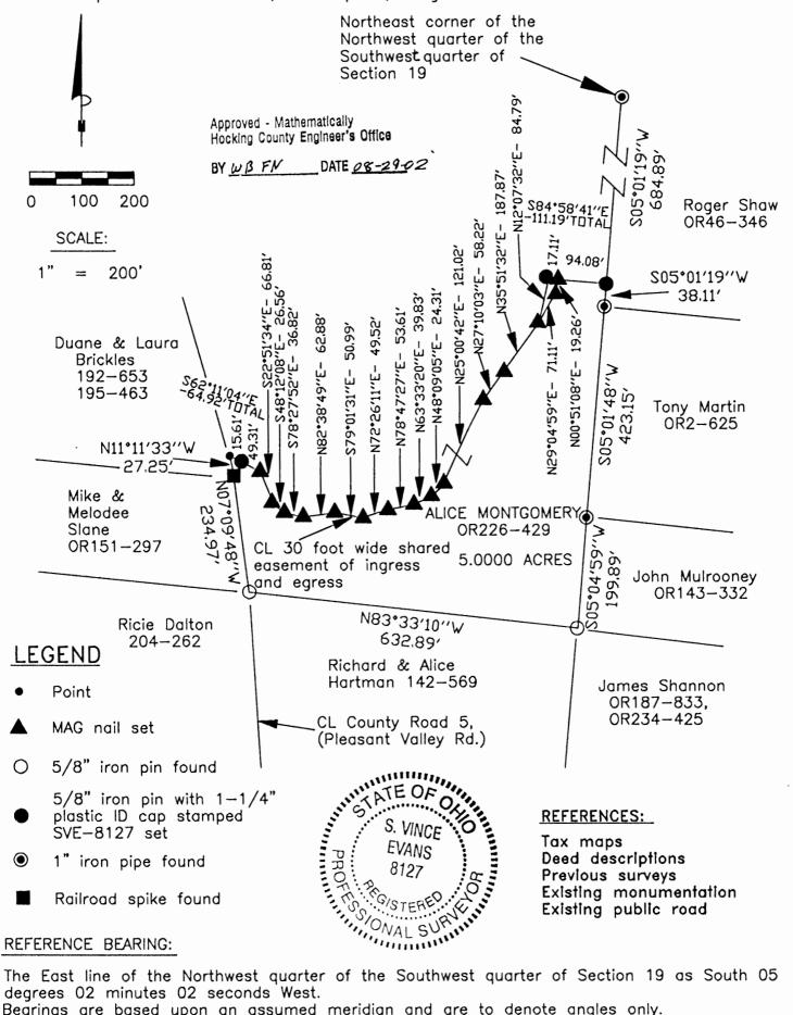
The East line of the Northwest quarter of the Southwest quarter of Section 19 as South 05 degrees 02 minutes 02 seconds West. Bearings are based upon an assumed meridian and are to denote angles only.
