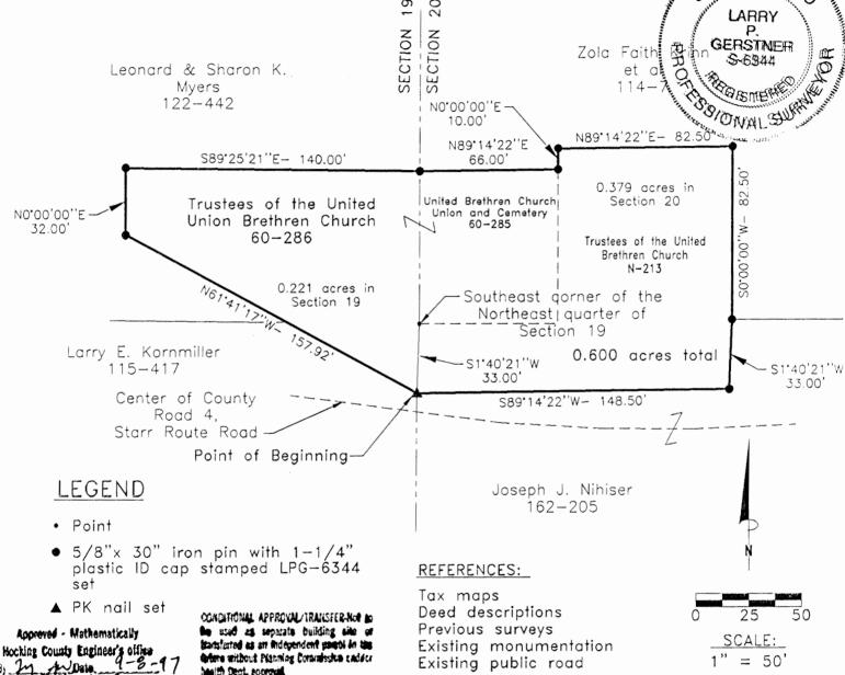
The East line of the Northeast quarter of Section 19 as North 0 degrees 00 minutes 00 seconds East. Bearings are based upon an assumed meridian and are to denote angles only.
