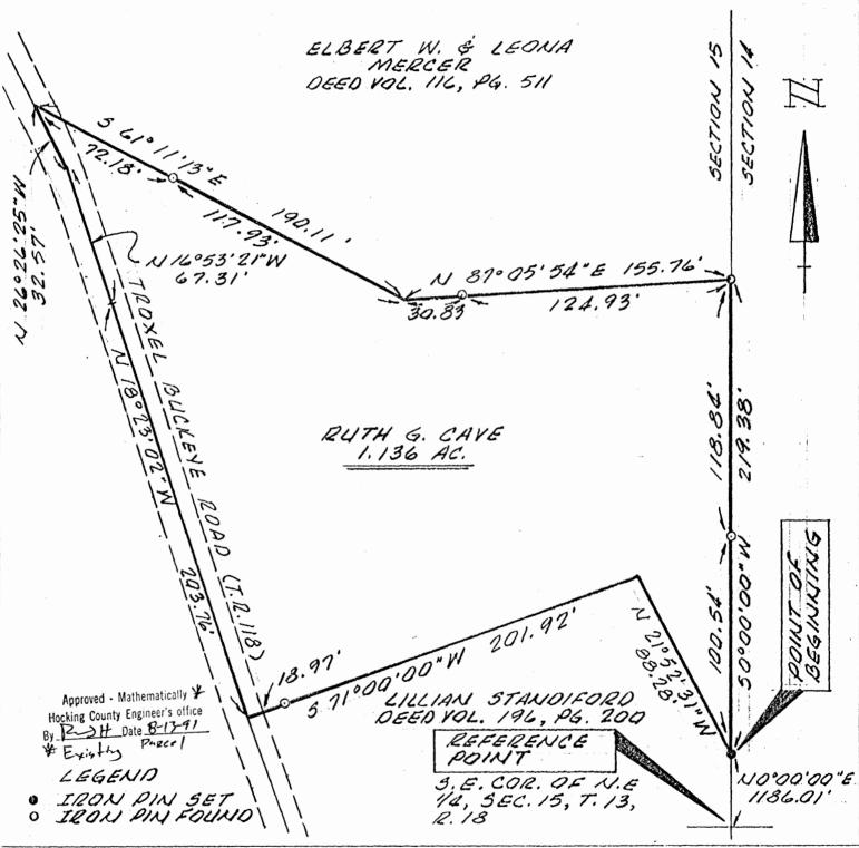
The bearing system for this plat is based on the east line of Section 15, Township 13, Range 18 as being N 0° 00' 00" E.
