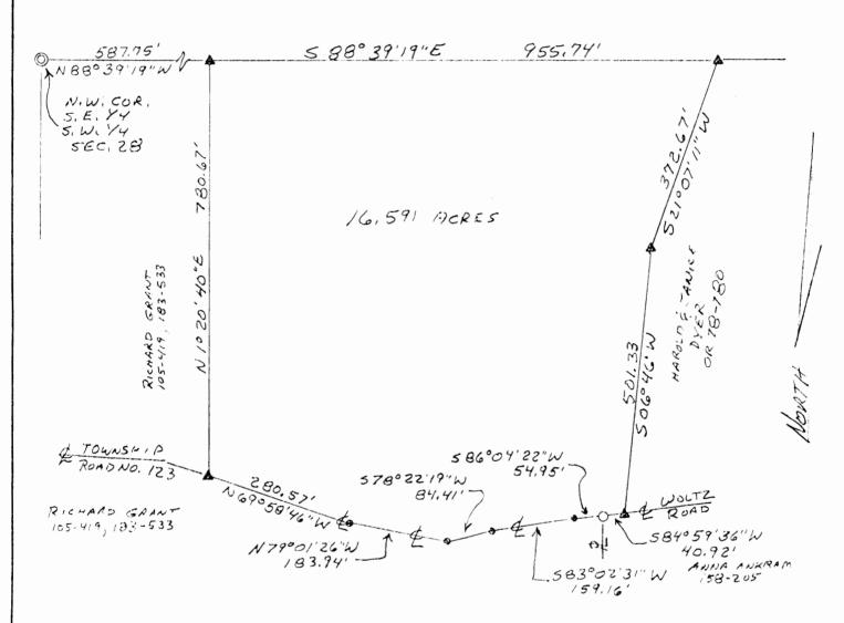
NOTE: BEARINGS DERIUED FROM MONUMENTS FOUND ON THE NORTH LINE OF THE S.W. MY OF THE S.E. MY OF SEC. 28 AS BEARING 388°39'19"E AND ARE FOR DETERMINATION OF ANGLES ONLY
