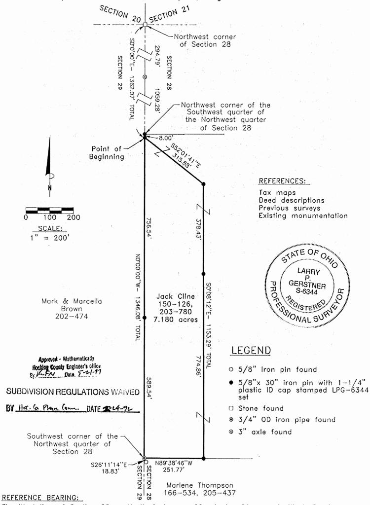
The West line of Section 28 as North 0 degrees 00 minutes 00 seconds West. Bearings are based upon an assumed meridian and are to denote angles only.
