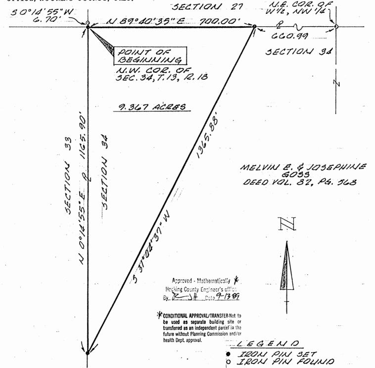
The bearing system for this plat is based on the west line of Section 34, Township 13, Range 18 as N 0° 14' 55" E.
