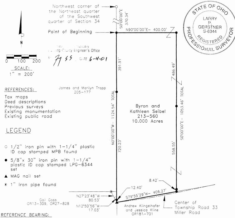
West line of the East half of the Southwest quarter of Section 34 as South 0 degrees 00 minutes 00 seconds East. Bearings are based upon an assumed meridian and are to denote angles only.
