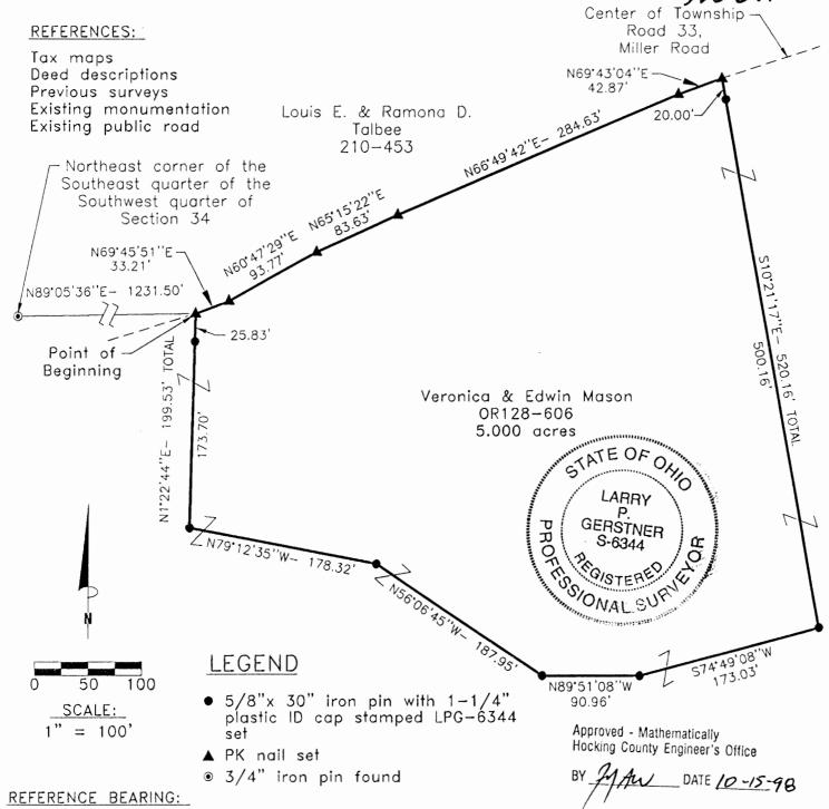
The North-South half Section line of Section 34 as North 4 degrées 41 minutes 40 seconds East. Bearings are based upon an assumed meridian and are to denote angles only.
