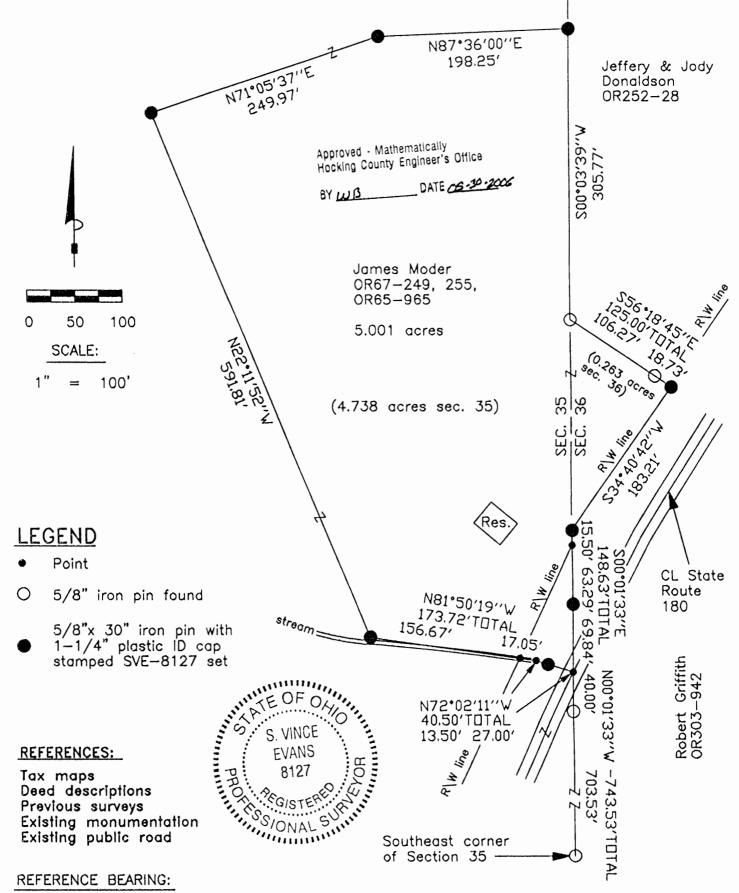
The east line of Section 35 as North 00 degrees 01 minutes 33 seconds West. Bearings are based upon an assumed meridian and are to denote angles only.
