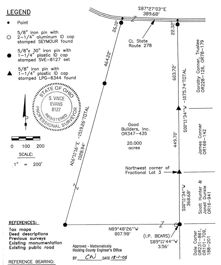
The South line of Fractional Lot 5 as North 89 degrees 28 minutes 08 seconds East. Bearings are based upon an assumed meridian and are to denote angles only.
