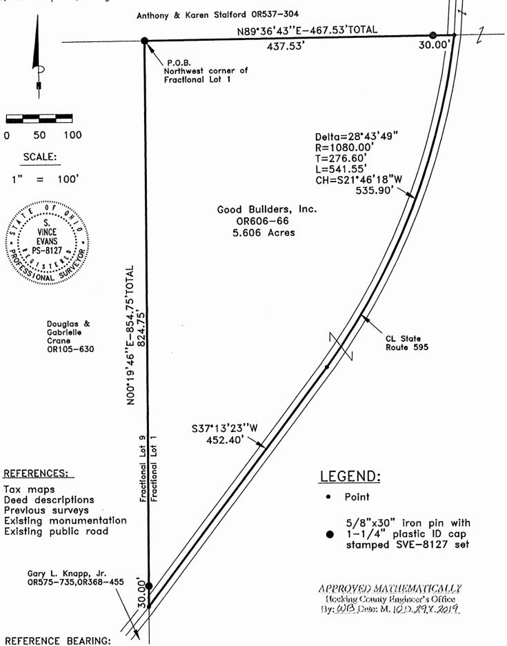
The north line of Fractional Lot 1 as North 89 degrees 36 minutes 43 seconds East. Bearings are based upon an assumed meridian and are to denote angles only.
