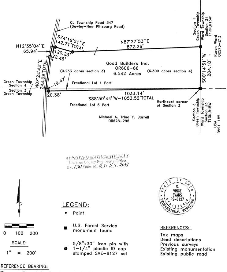
The east line of Section 4 as South 00 degrees 14 minutes 51 seconds West. Bearings are based upon an assumed meridian and are to denote angles only.
