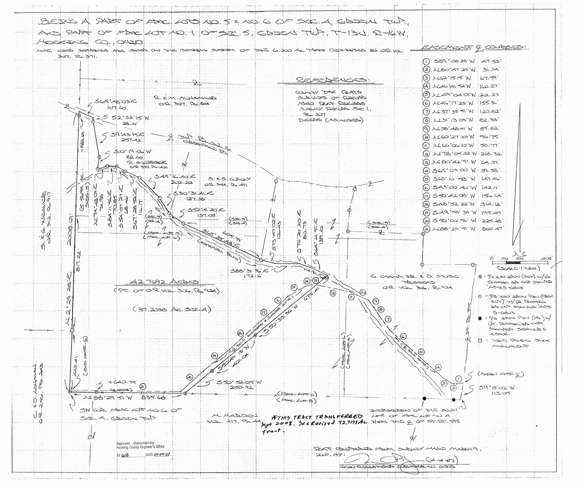
Being a non-exclusive 30.0 ft. wide easement for the purpose of ingress and egress across part of tracts described in O.R. Vol. 306, Pg. 924, situated in Frac. Lots No. 4 and No. 6 of Sec. 4, Green Twp., T-13N, R-16W, Hocking Co., Ohio. The centerline of said easement is described as follows:
