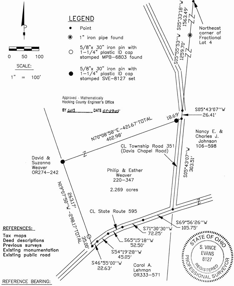
The East line of Fractional Lot 4 at this tract as South 05 degrees 43 minutes 07 seconds West. Bearings are based upon an assumed meridian and are to denote angles only.
