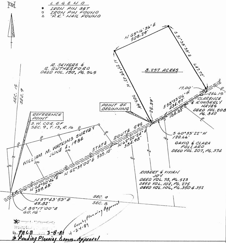
The bearing system for this plat is based on a previous survey by William M. Watkins dated June 4, 1984 on file at the Office of the Hocking County Engineer, Logan, Ohio.
