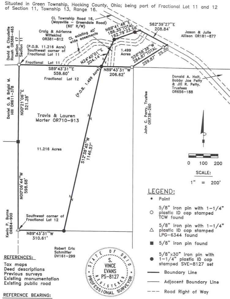
The south line of Fractional Lot 11 as South 89 degrees 43 minutes 31 seconds East. Bearings are based upon an assumed meridian and are to denote angles only. **CERTIFICATION:**
