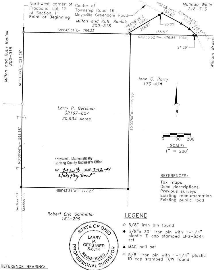
North line of Fractional Lot 12 of Section 11 as South 89 degrees 43 minutes 31 seconds East. Bearings are based upon an assumed meridian and are to denote angles only.
