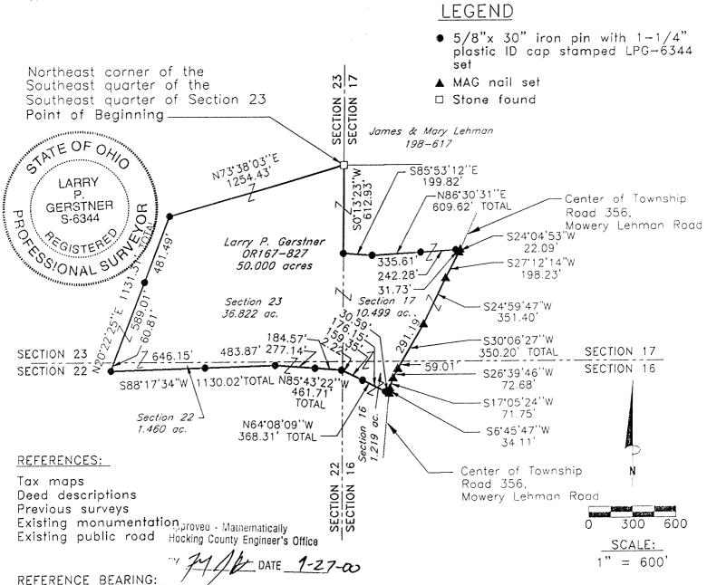
North line of Section 16 as North 90 degrees 00 minutes 00 seconds East. Bearings are based upon an assumed meridian and are to denote angles only.
