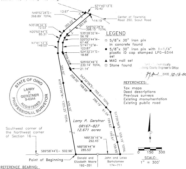
West line of Section 16 as North 0 degrees 13 minutes 23 seconds East. Bearings are based upon an assumed meridian and are to denote angles only.
