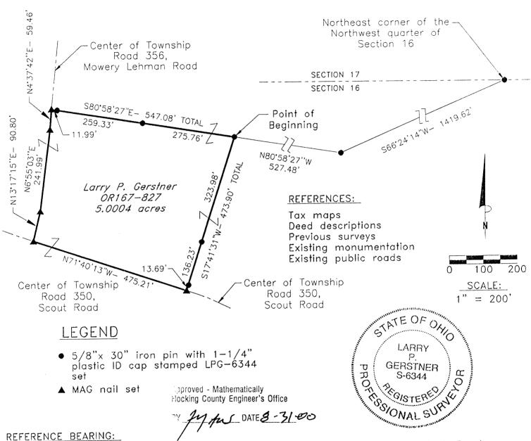
The North line of Section 16 as North 90 degrees 00 minutes 00 seconds East. Bearings are based upon an assumed meridian and are to denote angles only.
