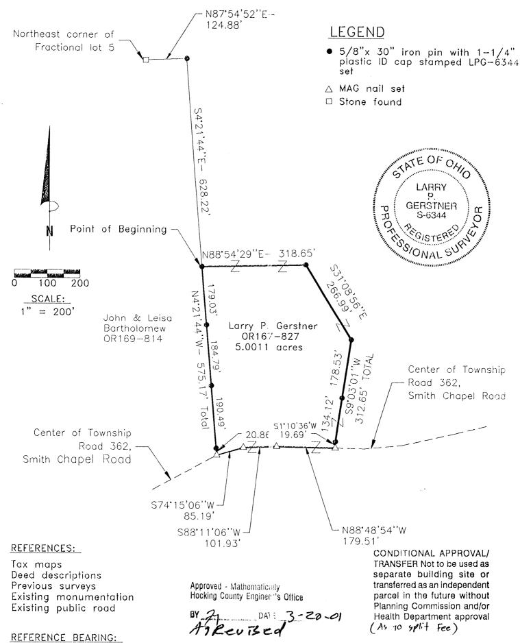
South line Section 16 as North 89 degrees 58 minutes 50 seconds West. Bearings are based upon an assumed meridian and are to denote angles only.
