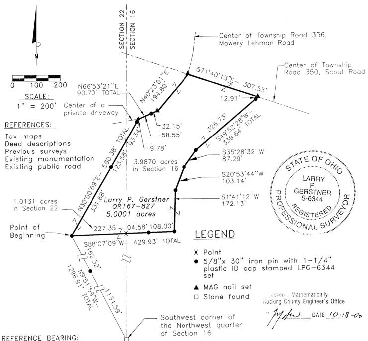
West line of Section 16 as North 0 degrees 13 minutes 23 seconds East. Bearings are based upon an assumed meridian and are to denote angles only.
