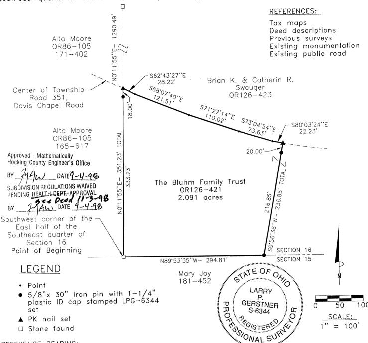
The West line of the East half of the Southeast quarter of Section 16 as North 0 degrees 11 minutes 55 seconds East. Bearings are based upon an assumed meridian and are to denote angles only.
