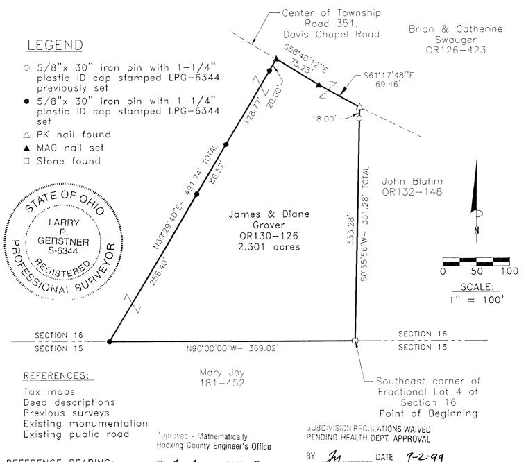
The South line of Section 16 as North 90 degrees 00 minutes 00 seconds West. Bearings are based upon an assumed meridian and are to denote angles only.
