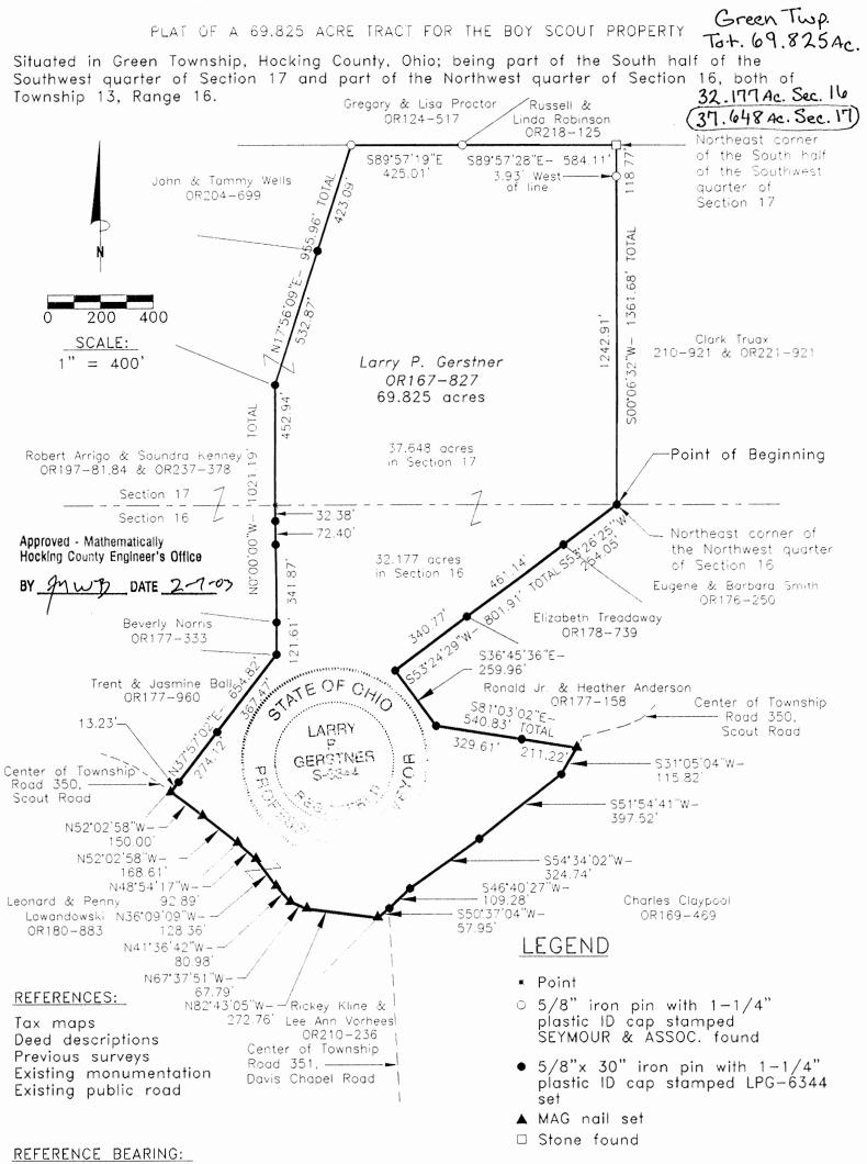
North line of Section 16 as North 90 degrees 00 minutes 00 seconds West. Bearings are based upon an assumed meridian and are to denote angles only.
