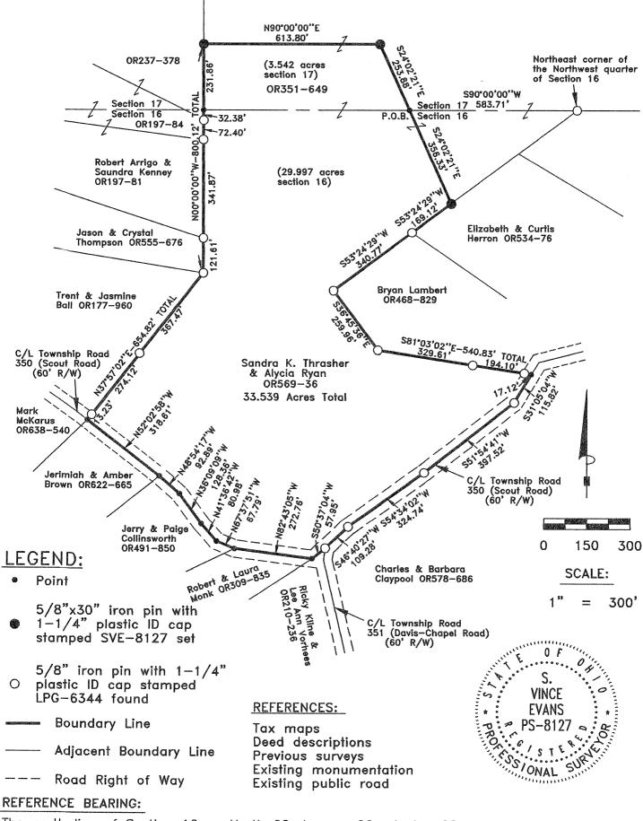
The north line of Section 16 as North 00 degrees 00 minutes 00 seconds West. Bearings are based upon an assumed meridian and are to denote angles only. **CERTIFICATION:**
