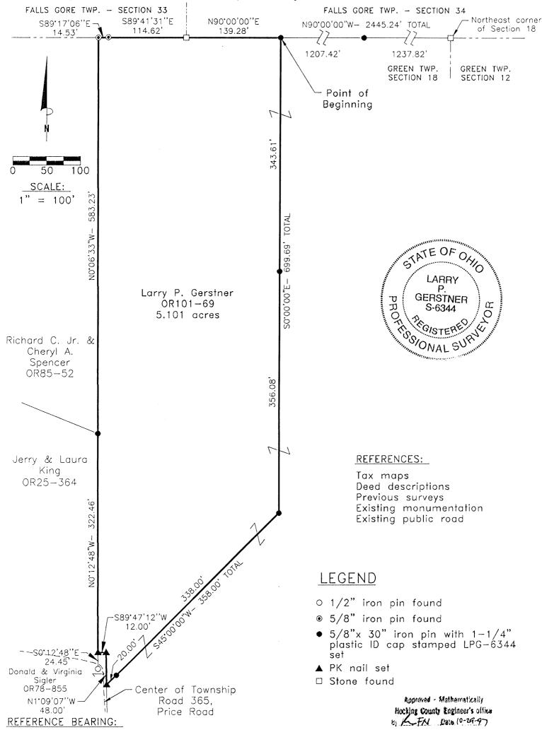
A portion of the North line of Section 18 as North 90 degrees 00 minutes 00 seconds West. Bearings are based upon an assumed meridian and are to denote angles only.
