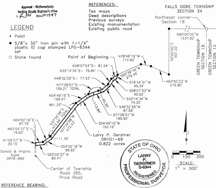
The North line of Section 18 as North 90 degrees 00 minutes 00 seconds West. Bearings are based upon an assumed meridian and are to denote angles only.
