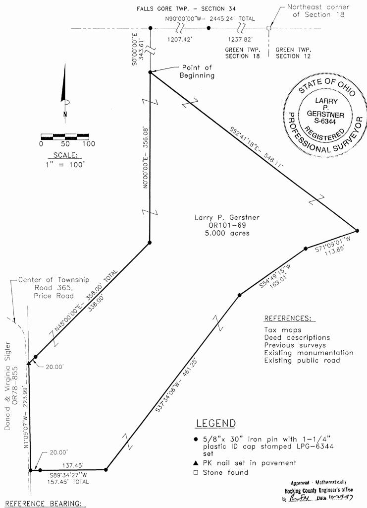
The North line of Section 18 as North 90 degrees 00 minutes 00 seconds West. Bearings are based upon an assumed meridian and are to denote angles only.
