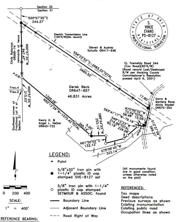
The east line of Fractional Lot 4 as North 00 degrees 57 minutes 35 seconds West. Bearings are based upon an assumed meridian and are to denote angles only.
