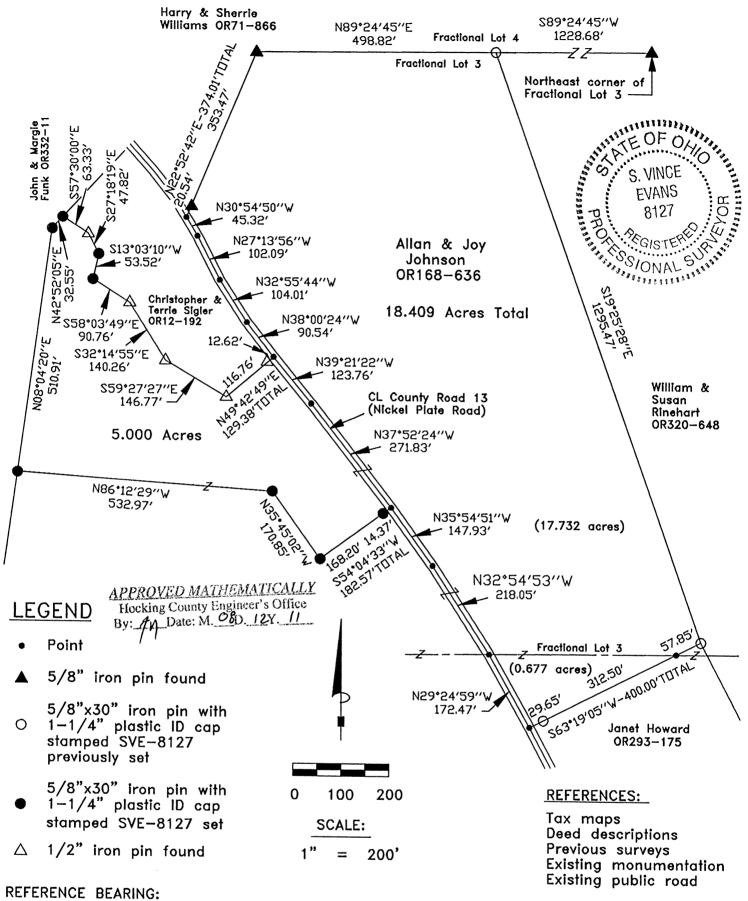
The East line of the Southwest quarter of Section 31 as South 00 degrees 00 minutes 00 seconds East. Bearings are based upon an assumed meridian and are to denote angles only.
