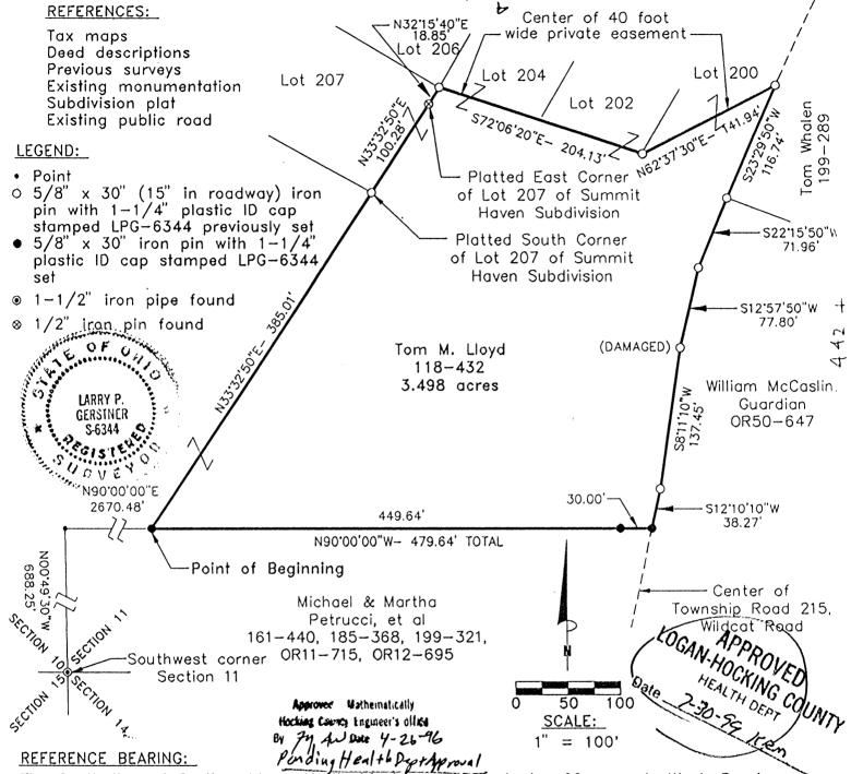
The South line of Section 11 as North 90 degrees 00 minutes 00 seconds West. Bearings are based upon an assumed meridian and are to denote angles only.
