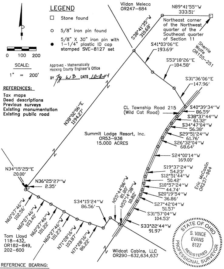
The West line of the Southwest quarter of the Northeast quarter of Section 11 as North 00 degrees 31 minutes 44 seconds East. Bearings are based upon an assumed meridian and are to denote angles only.
