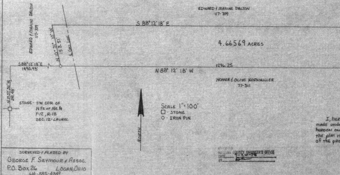
OTTO A. SHHWI 91-115 a 1370.32 5 0° 56' 20'W 043,57 1339.82' E Co Rd 5. I, here by certify that AN ACTUAL SURVEY WAS made under my supervision of the premises shown hereon on the 23rd day of September, 1978; that the plat is a true and correct representation of the premises as determined by said survey. 1. Seymon OHIO REDISTERED SURVEYOR NO. 6044
