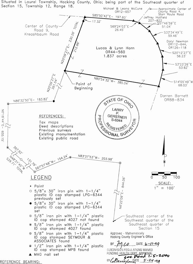
The West line of a 2.00 acre survey by registered surveyor no. 4027 as South 6 degrees 22 minutes 09 seconds West. Bearings are based upon an assumed meridian and are to denote angles only.
