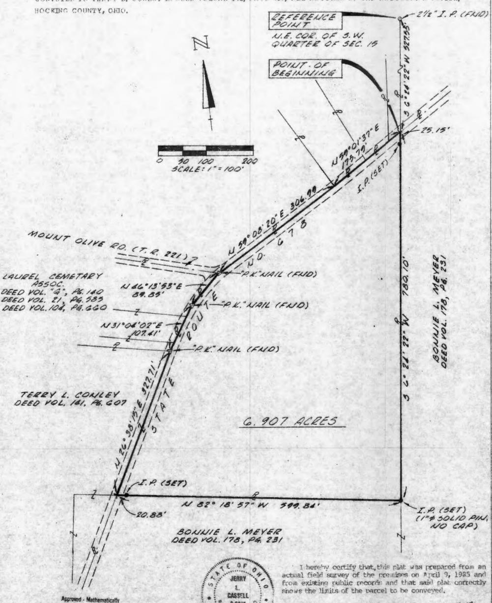
The bearing system for this plat is based on transit compass needle bearings, adjusted for local declination, observed on survey traverse courses.
