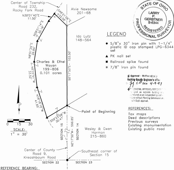
The East line of Section 15 as North 0 degrees 17 minutes 50 seconds West. Bearings are based upon an assumed meridian and are to denote angles only.
