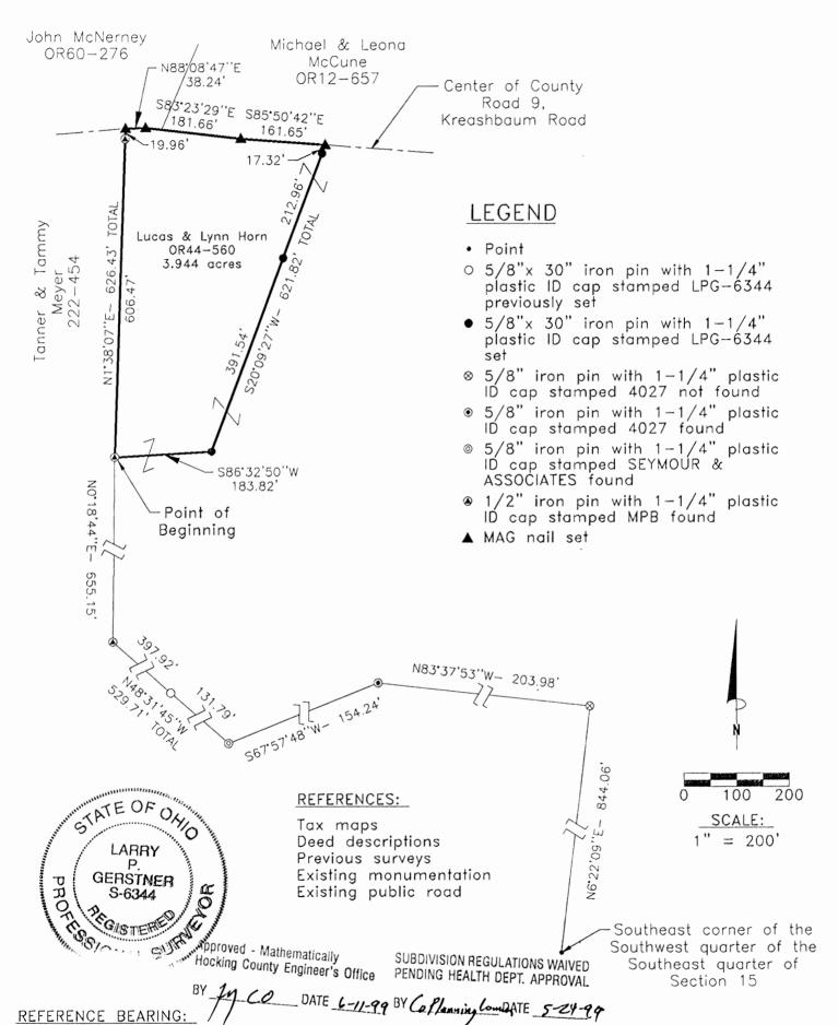
The West line of a 2.00 acre survey by registered surveyor no. 4027 as South 6 degrees 22 minutes 09 seconds West. Bearings are based upon an assumed meridian and are to denote angles only.
