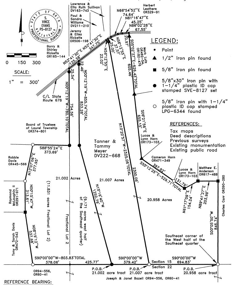
The south line of Section 15 as South 90 degrees 00 minutes 00 seconds West. Bearings are based upon an assumed meridian and are to denote angles only.
