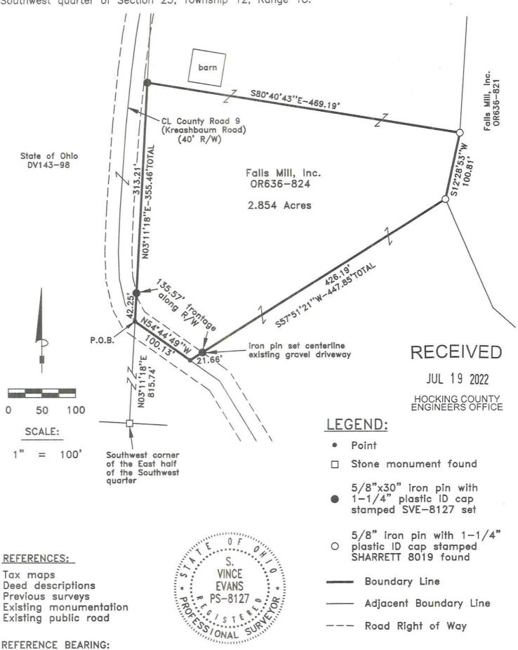
The west line of the East half of the Southwest quarter as North 03 degrees 11 minutes 18 seconds East. Bearings are based upon an assumed meridian and are to denote angles only.
