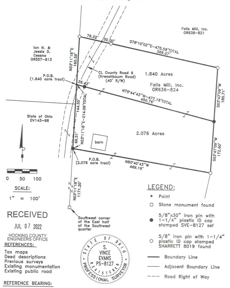
The west line of the East half of the Southwest quarter as North 03 degrees 11 minutes 18 seconds East. Bearings are based upon an assumed meridian and are to denote angles only.
