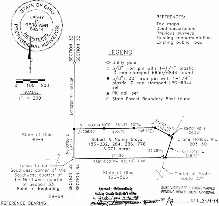
The West line of Section 33 as North 0 dégrees 00 minutes 00 seconds East. Bearings are based upon an assumed meridian and are to denote angles only.
