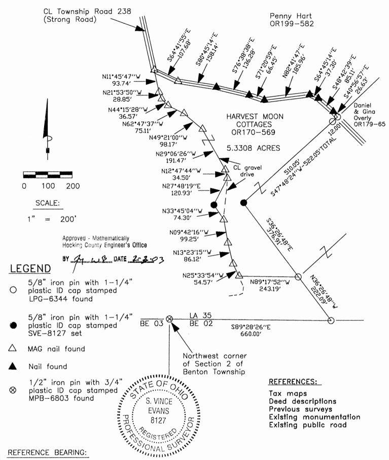
The South line of Section 35 as South 89 degrees 28 minutes 26 seconds East. Bearings are based upon an assumed meridian and are to denote angles only.
