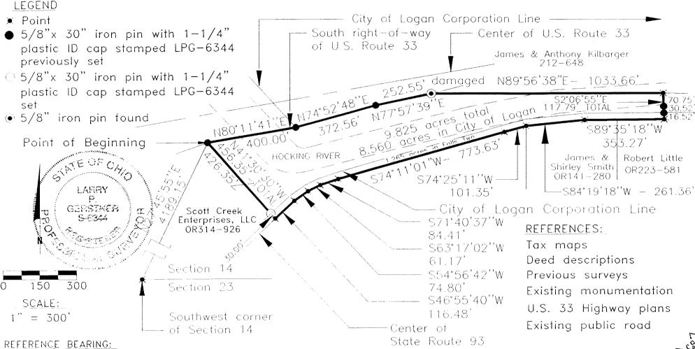
South line of Section 14 as North 90 degrees 00 minutes 00 seconds East. Bearings are based upon an assumed meridian and are to denote angles only.
