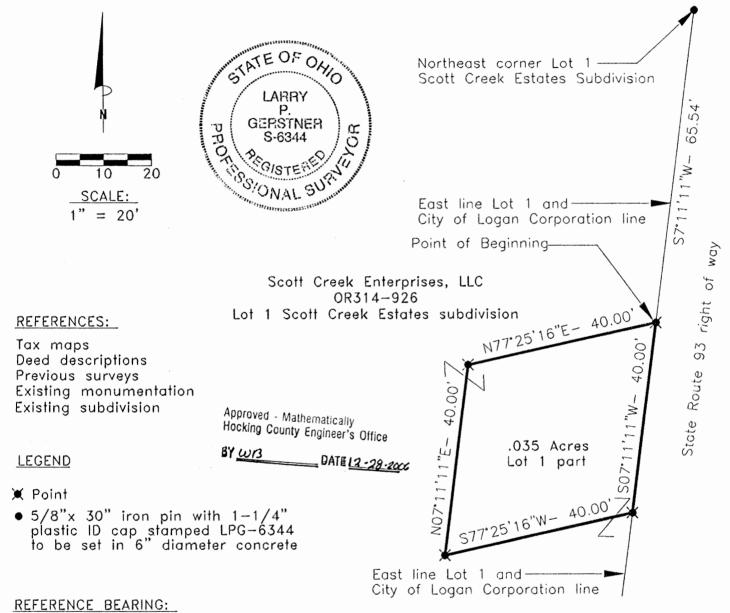
The South line of Lot 1 as South 7 degrees 11 minutes 11 seconds West. Bearings are based upon an assumed meridian and are to denote angles only.
