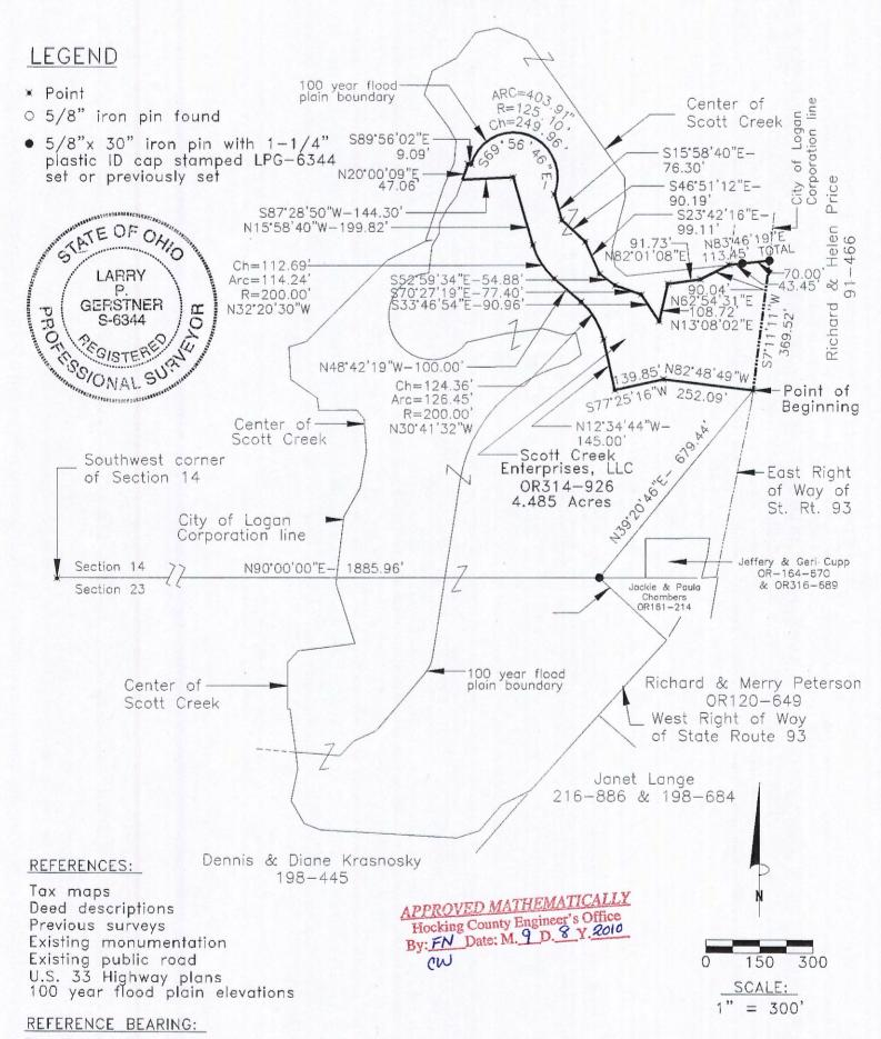
The South line of Section 14 as North 90 degrees 00 minutes 00 seconds East. Bearings are based upon an assumed meridian and are to denote angles only.
