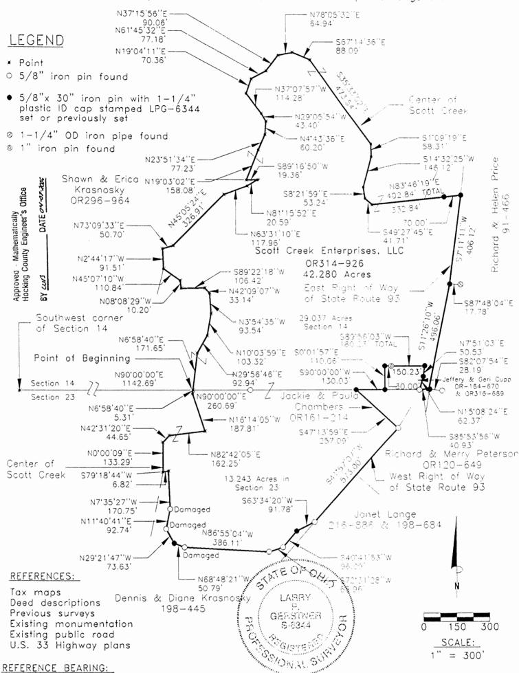
The South line of Section 14 as North 90 degrees 00 minutes 00 seconds East. Bearings are based upon an assumed meridian and are to denote angles only.
