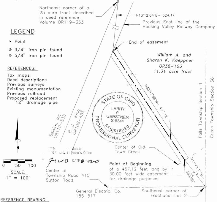
East line of Fractional Lot 2 as North 0 degrees 00 minutes 00 seconds East. Bearings are based upon an assumed meridian and are to denote angles only.
