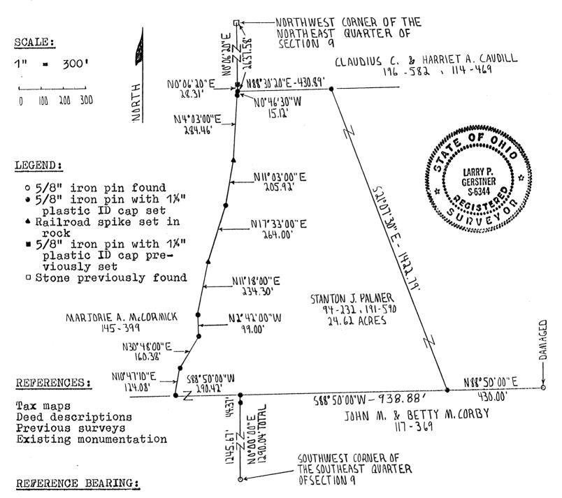
The North - South half Section line of Section 9 as North 0 degrees 00 minutes 00 seconds East.
