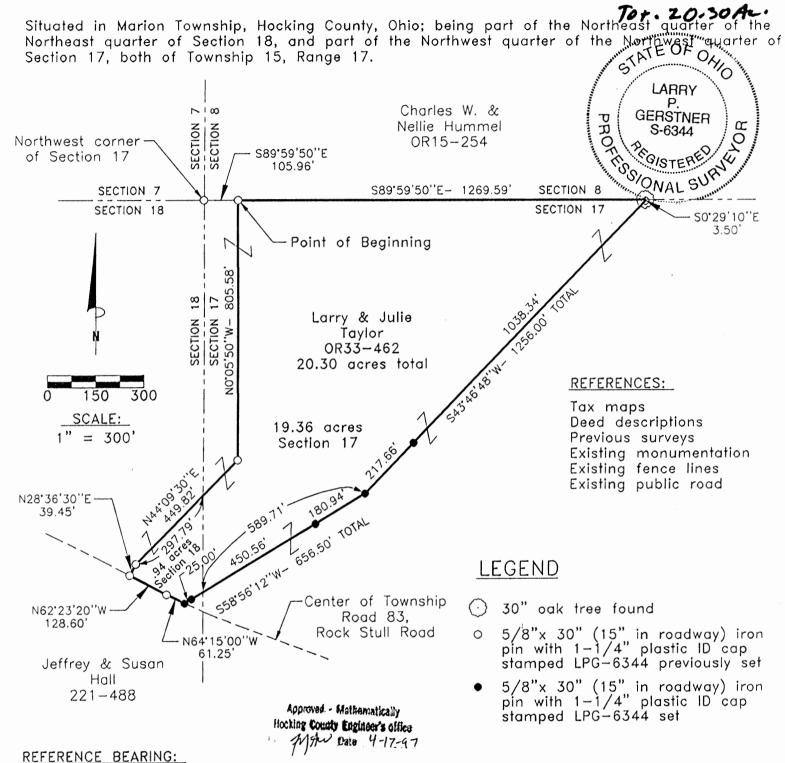
The North line of Section 17 as South 89 degrees 59 minutes 50 seconds East. Bearings are based upon an assumed meridian and are to denote angles only.
