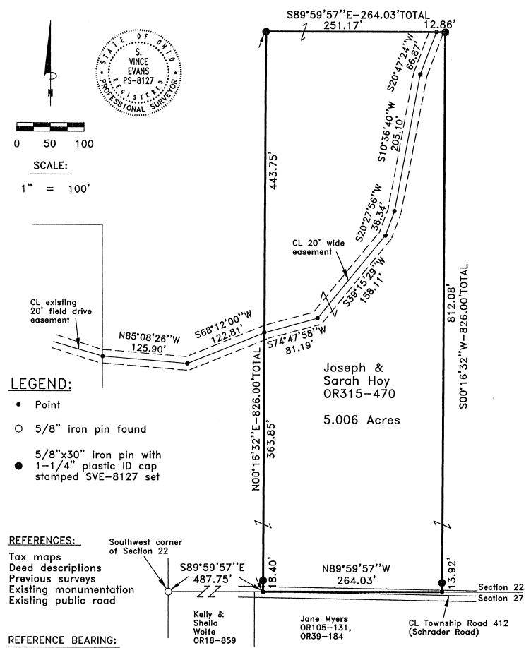
The south line of Section 22 as South 89 degrees 59 minutes 57 seconds East. Bearings are based upon an assumed meridian and are to denote angles only.
