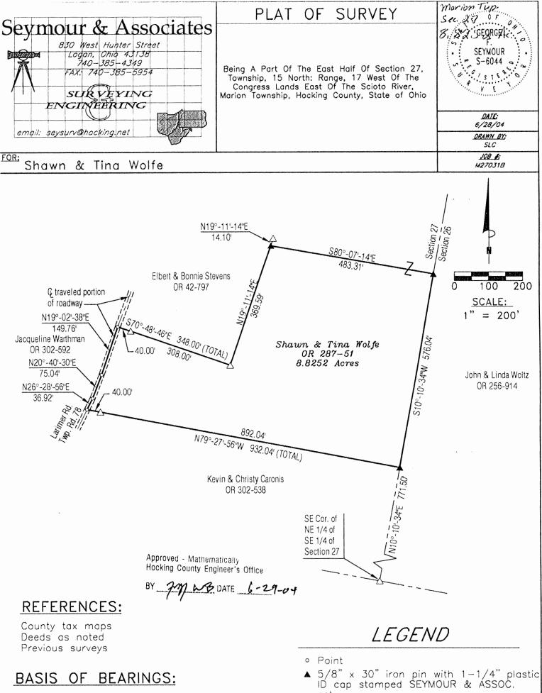
Bearings derived from monumentation found on the East line of Section 27 as bearing South 10 degrees 10 minutes 34 seconds West and are for the determination of angles only.
