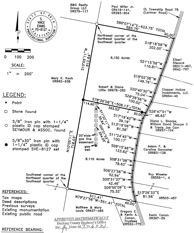
The west line of the Northeast quarter of the Southeast quarter as North 10 degrees 05 minutes 11 seconds East. Bearings are based upon an assumed meridian and are to denote angles only.
