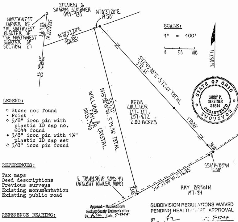
A previous survey by registered surveyor no. 753 done June 30, 1967 making the West line of Section 27 South 6 degrees 00 minutes 00 seconds West.
