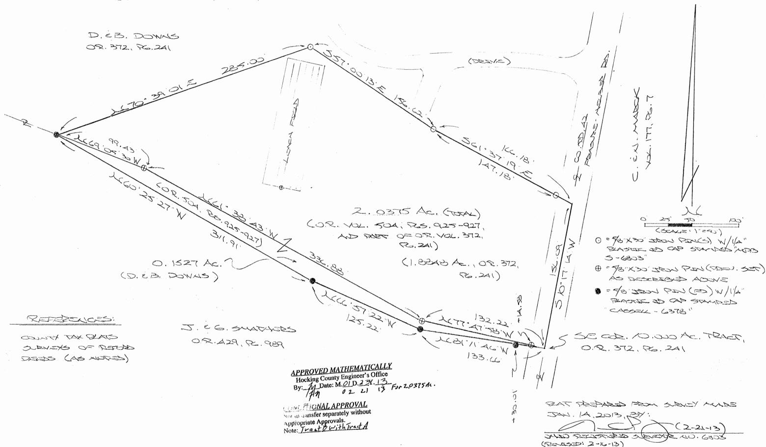
Being the 0.1527 Ac. tract described in Vol. 504, Pgs. 925-927, Hocking Co. Official Records, and part of the 10.000 Ac. tract described in O.R. Vol. 372, Pg. 241, situated in the NW \(^1\)4 of Sec. 34 Marion Twp., T-15N, R-17W, Hocking Co., Ohio, and being more particularly described as follows:
