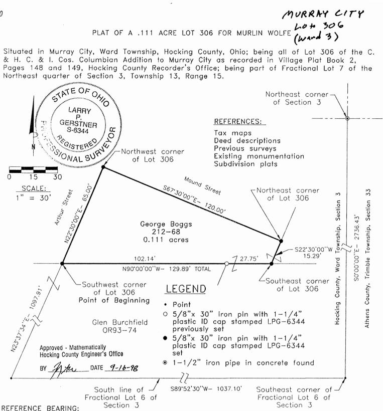
The East line of Section 3 as South 0 degrees 00 minutes 00 seconds East. Bearings are based upon an assumed meridian and are to denote angles only.
