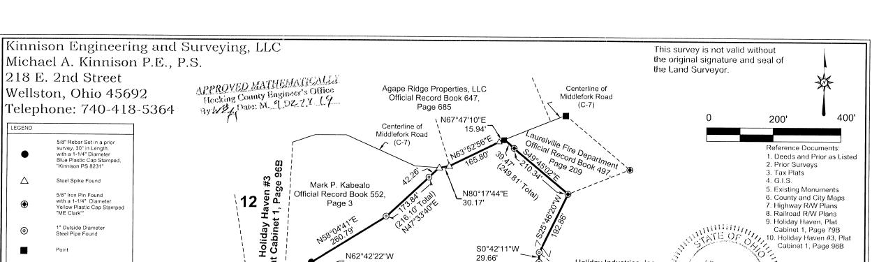
1" Outside Diameter 0 Steel Pipe Found 5/8" Iron Pin Found, No Cap or Tag 5/8" Iron Pin Found with 1-1/4" Diameter 0 Red Cap Stamped "Mike Clark PLS 6808" 5/8" Rebar Set, 30" in Length with a 1-1/4" Diameter Blue Plastic Cap Stamped, "Kinison PS 8231"
