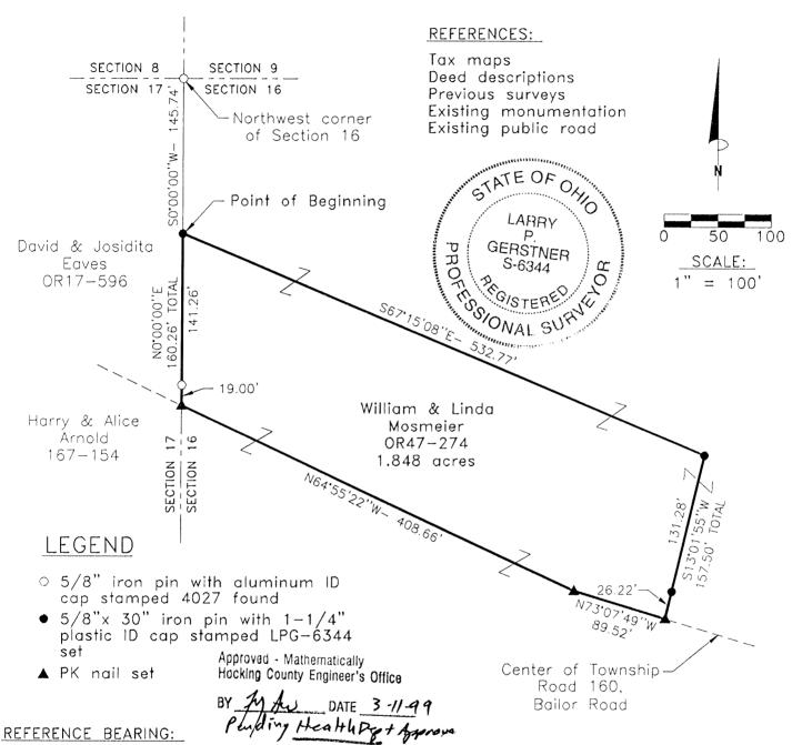
The West line of Section 16 as North 0 degrees 00 minutes 00 seconds East. Bearings are based upon an assumed meridian and are to denote angles only.
