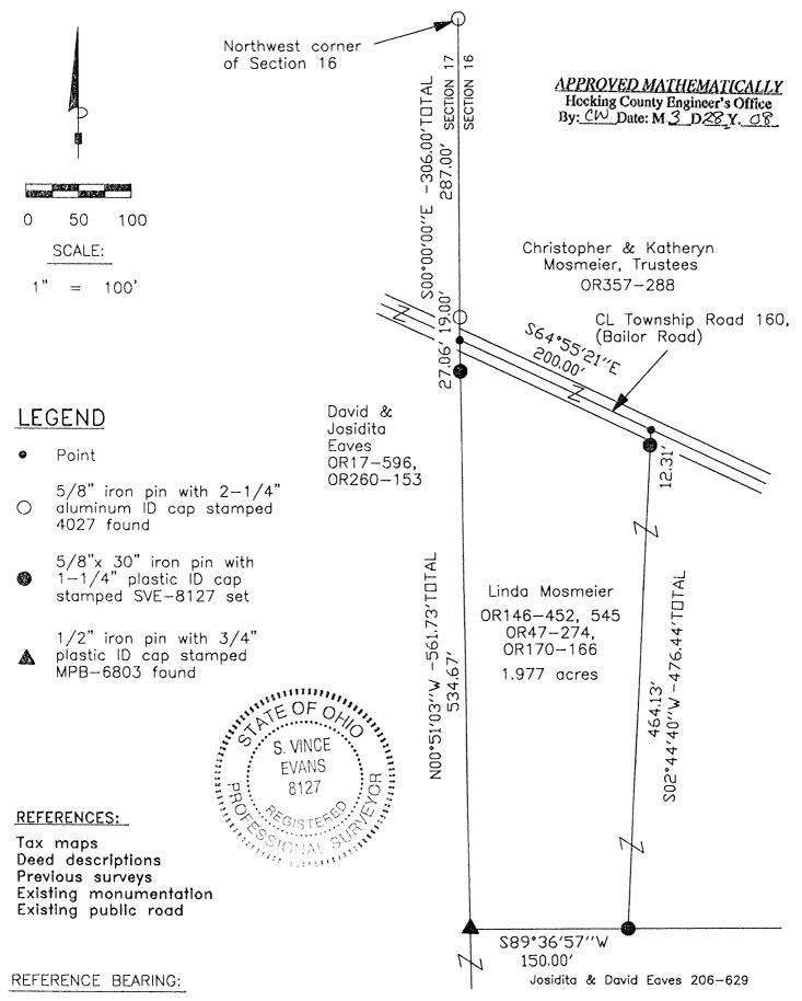
The West line of Section 16 as South 00 degrees 00 minutes 00 seconds East. Bearings are based upon an assumed meridian and are to denote angles only.
