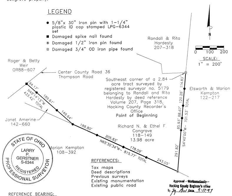
The May 5, 1986 survey by registered surveyor no. 6803 making the South line of this tract North 65 degrees 30 minutes 34 seconds West. Bearings are based upon an assumed meridian and are to denote angles only.
