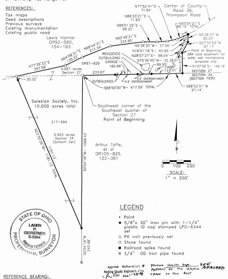
The West line of Section 34 (bottom tier) as North 0 degrees 00 minutes 00 seconds East. Bearings are based upon an assumed meridian and are to denote angles only.
