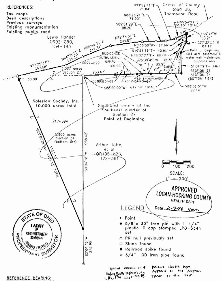
The West line of Section 34 (bottom tier) as North 0 degrees 00 minutes 00 seconds East. Bearings are based upon an assumed meridian and are to denote angles only.
