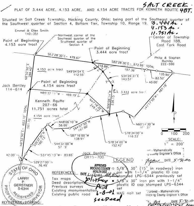
The North line of Section 4 Bottom Tier as South 82 degrees 28 minutes 30 seconds Bearings are based upon an assumed meridian and are to denote angles only.
