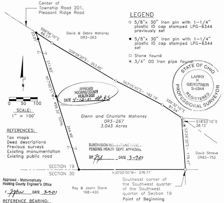
South line of Section 19 as North 90 degrees 00 minutes 00 seconds West. Bearings are based upon an assumed meridian and are to denote angles only.
