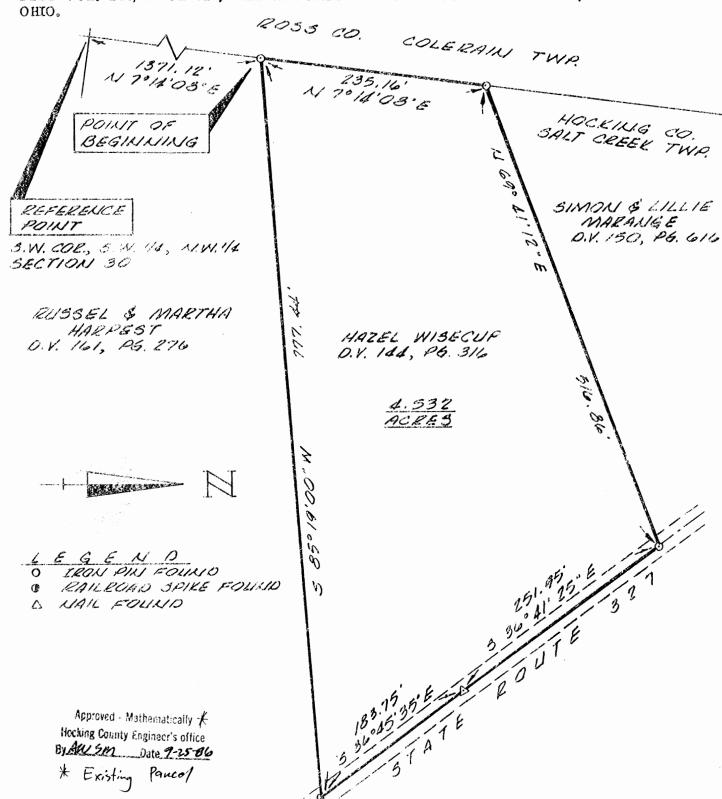
The bearing system for this plat is based on the Russel and Martha Harpest parcel as recorded in Deed Vol. 161, Page 276.
