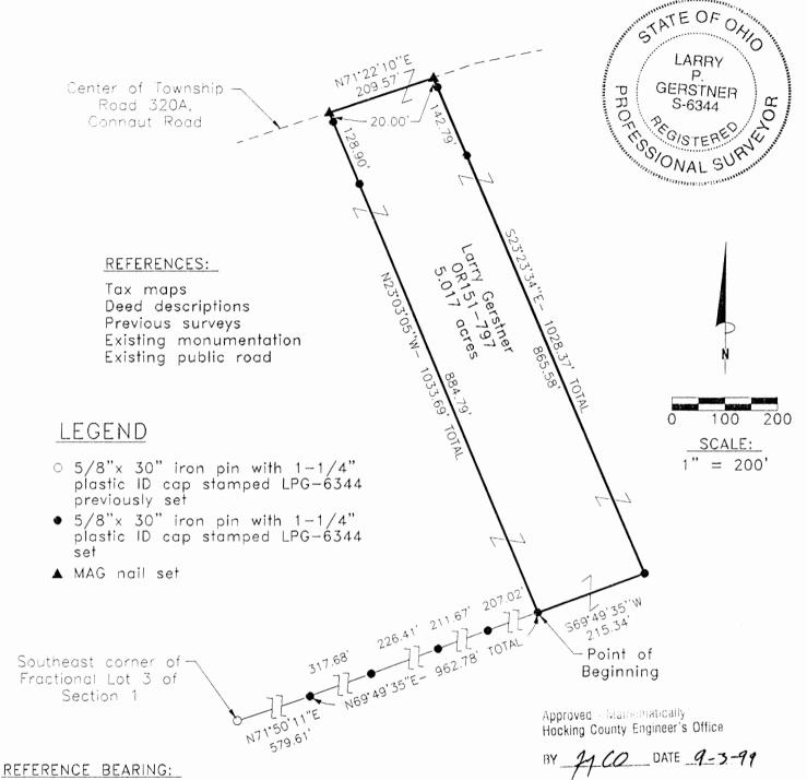
The West line of Section 2 of Starr Township as North 0 degrees 00 minutes 00 seconds East. Bearings are based upon an assumed meridian and are to denote angles only.
