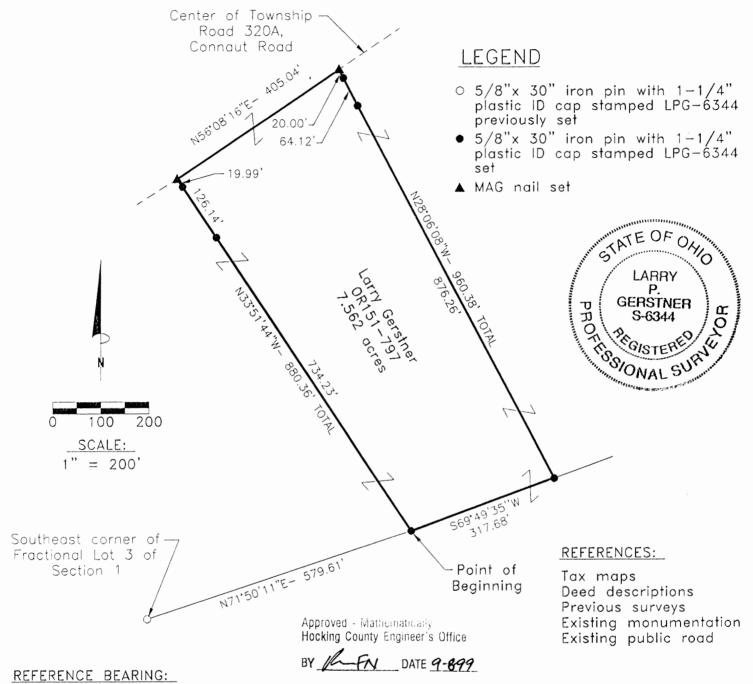
The West line of Section 2 of Starr Township as North 0 degrees 00 minutes 00 seconds East. Bearings are based upon an assumed meridian and are to denote angles only.
