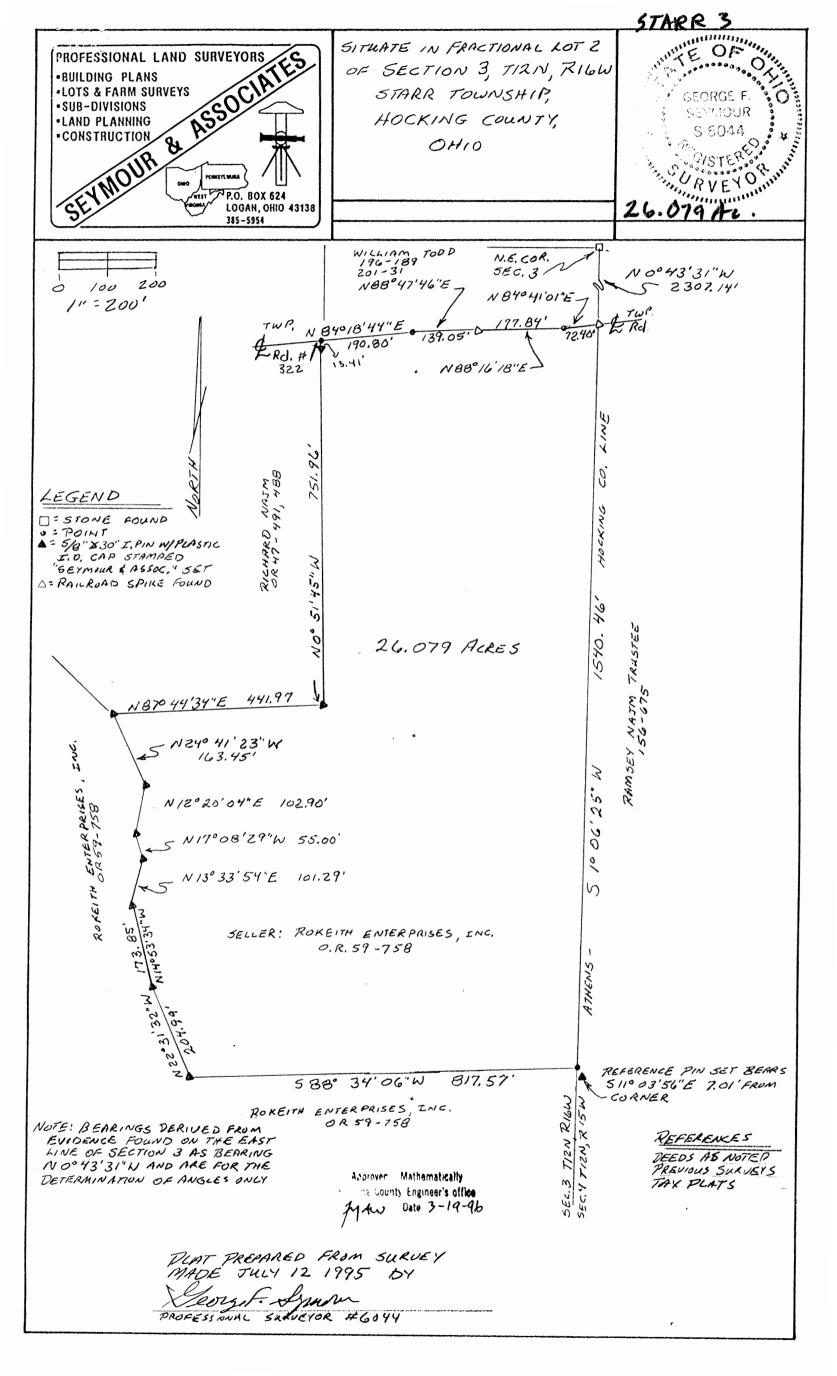
Being a part of the tract of land that is now or formerly in the name of Rokeith Enterprises, Inc. as recorded in Official Record 59 at page 758, Hocking County Recorder's Office, said tract being part of Fractional Lot 2 in Section 3, T12N, R16W, Starr Township, Hocking County, State of Ohio and being more particularly described as follows:
