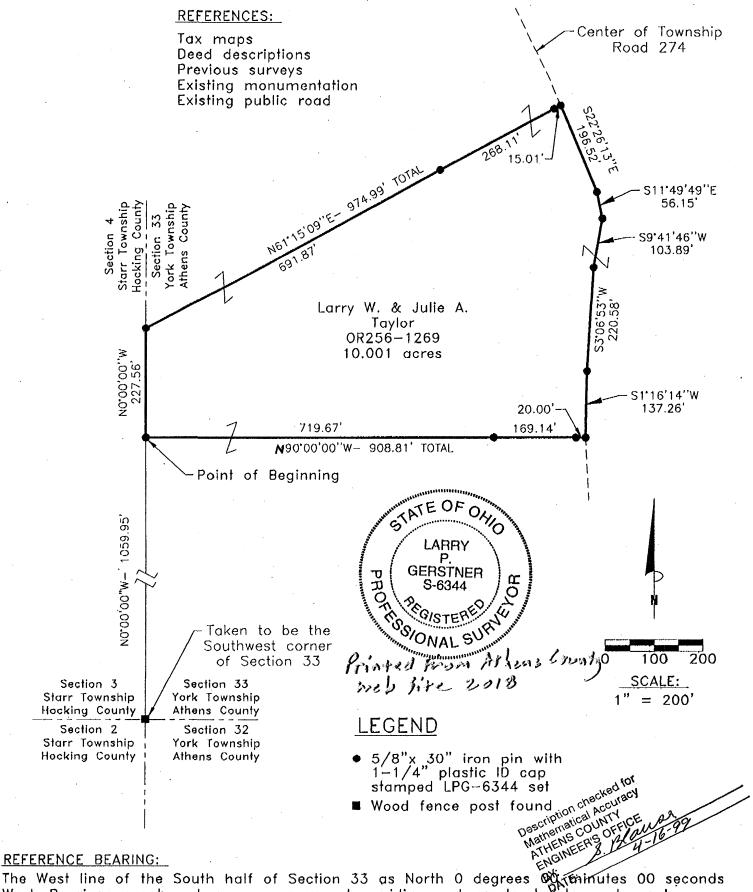
The West line of the South half of Section 33 as North 0 degrees of the inutes 00 seconds West. Bearings are based upon an assumed meridian and are to denote angles only.
