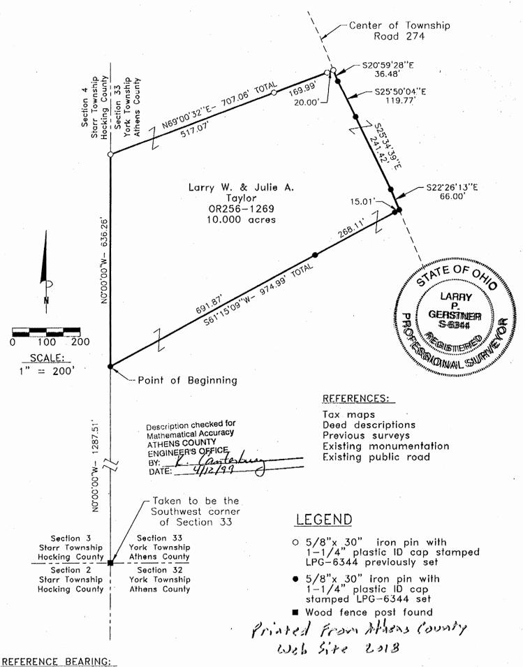
The West line of the South half of Section 33 as North 0 degrees 00 minutes 00 seconds West. Bearings are based upon an assumed meridian and are to denote angles only.
