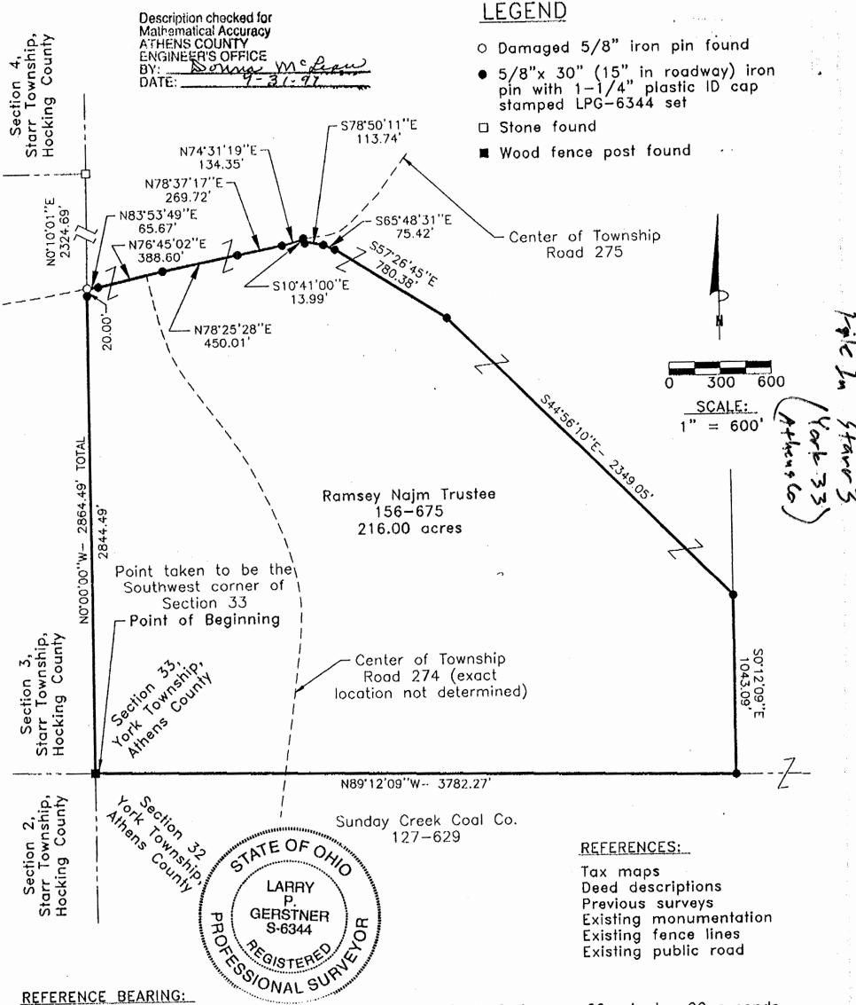
The West line of the South half of Section 33 as North 0 degrees 00 minutes 00 seconds West. Bearings are based upon an assumed meridian and are to denote angles only.
