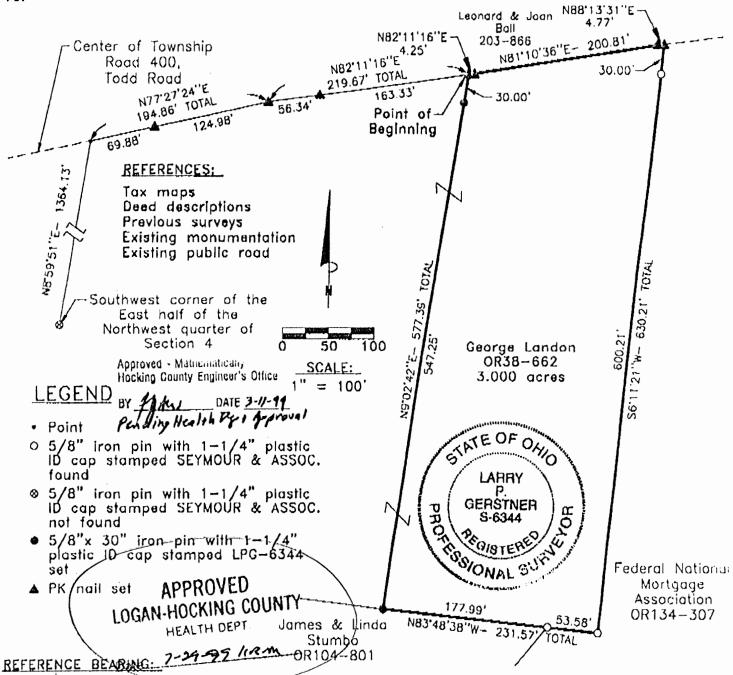
The West line of the East half of the Northwest quarter of Section 4 as North 8 degrees 59 minutes 51 seconds East. Bearings are based upon an assumed meridian and are to denote angles only.
