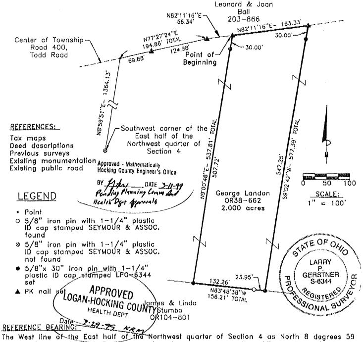
The West line of the East half of the Northwest quarter of Section 4 as North 8 degrees 59 minutes 51 seconds East. Bearings are based upon an assumed meridian and are to denote angles only.
