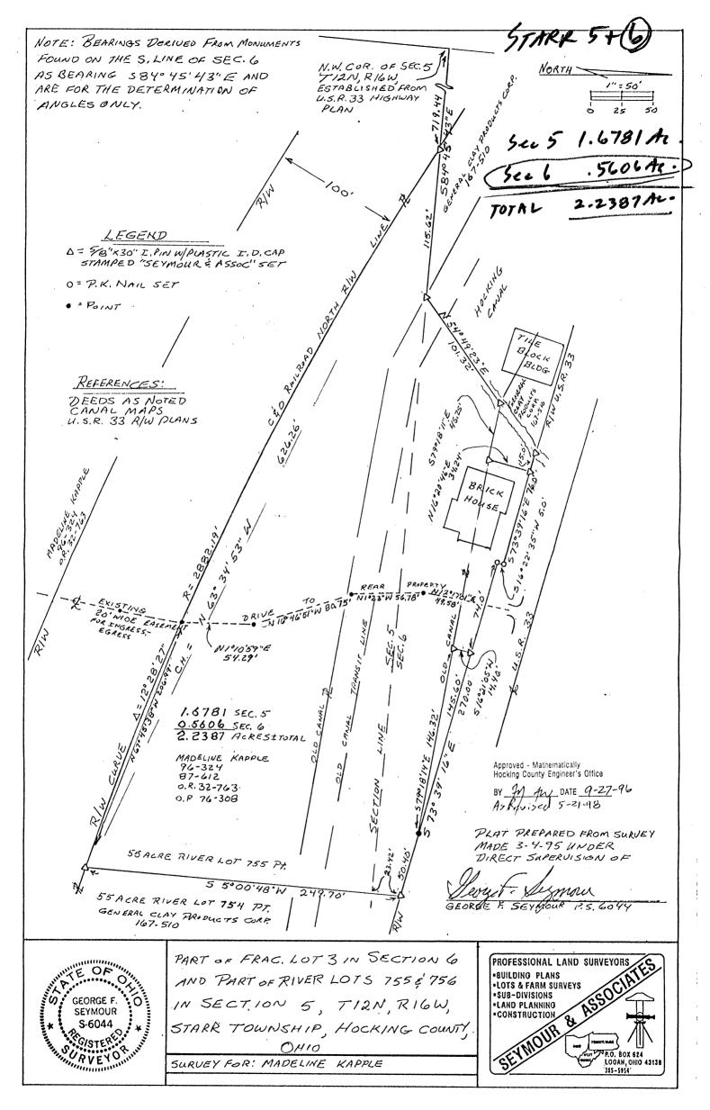
Thence leaving said right of way line, South 05 degrees 00 minutes 48 seconds West, crossing into Section 5 at 23.42 feet, going a total distance of 249.70 feet to a 5/8" X 30" iron pin with a plastic identification cap set on the northerly property line of C & O Railroad;
