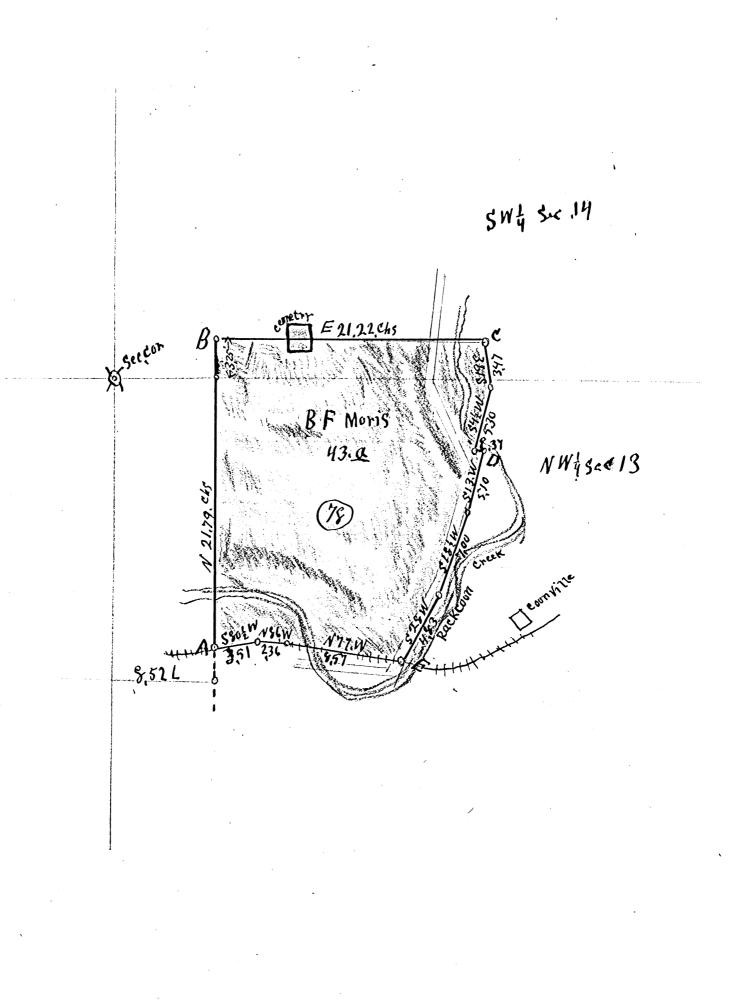
A otes to Surveys in Sec No 135 14 TP 12 RIG. Sum Ston Belging at A: in Centin of RR There to B W. oak 14 S32 W 34 kindes W. oak S' S69 E 12 links C=Elm 12" S 1.00 E 1.43 L D= Elm 24 N 18, E. 8 L Woole 40 N 23, W 30, L 18 F= centre of RR a Grc\_30. N434 & So.L Centify the foregoing to Be a true copy of Survey mod By me fm BFE Minis Jan 22, 1906 Eph Show, Surveyon FROM RECORD OF SURVEYS BOOK #1 PAGE 136+137 HOCKING COUNTY ENGINEERS OFFICE
