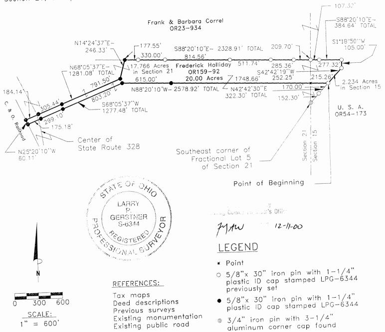
East line of Section 21 as South 0 degrees 48 minutes 50 seconds West. Bearings are based upon an assumed meridian and are to denote angles only.
